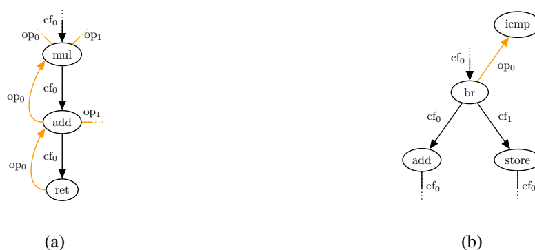
Figure 5.3: Graph representation of control-flow transition for non-diverting instructions (a) and br instructions (b).
