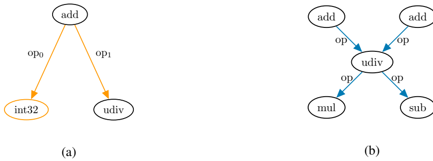
Figure 5.1: Graph representation of an add instruction (a) and an ambiguous, and therefore rejected, representation of instructions with variable operand counts (b).
