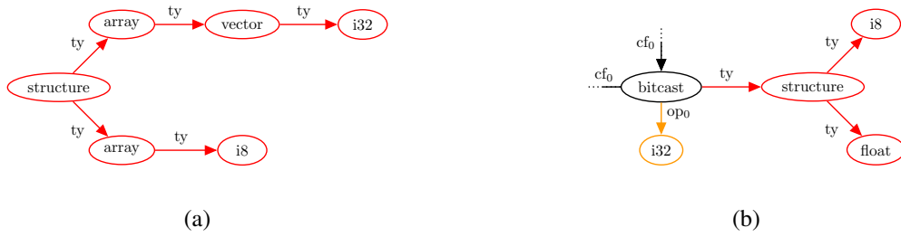
Figure 5.6: Graph representation of structure declaration (a) and a bitcast instruction utilizing a previously declared structure as target type (b).
