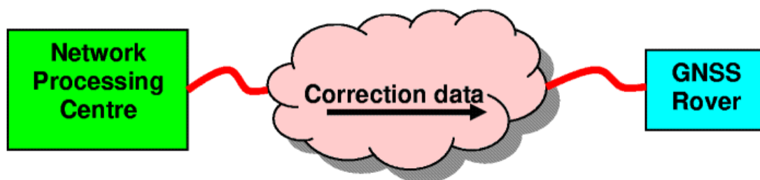
Fig. 3: Communication in simplex operating mode.
