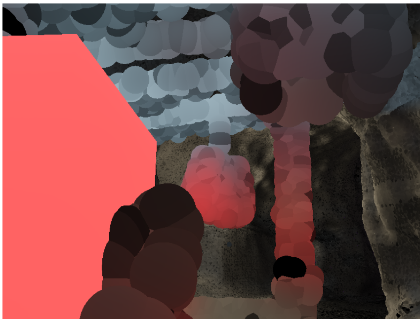
Figure 4.1: A section of a scene that consists of a large point cloud rendered with spherical surfels and a pink emissive cube rendered as a triangle based mesh.
