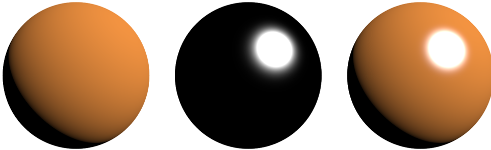
Figure 2.3: A non-metallic sphere of brown albedo illuminated from the top-right by a white light source. From left to right: diffuse reflections, glossy reflections resulting in a highlight, and the combined effect of both. Note that these images are only intended to outline the different effects and are not physically correct rendered.
