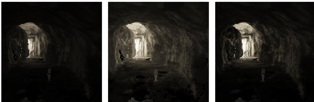
Figure 5.3: Albedo adjustment. Left to right: no adjustment, with albedo adjustment of 0.33, with adjustment but only a single bounce (note how little light reaches the floor in the foreground).
