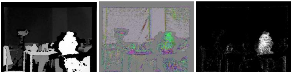
Figure 3.2: A visualization of the intermediate output of the random forest. Left: The depthmap of the scene. E^{depth}(H) uses the depthmap to verify the pose hypothesis. Middle: The prediction image of the object coordinates. The object coordinates are mapped to the color cube. E^{coord}(H) penalizes the deviation of the inferred object coordinates to rendered object coordinates of the pose H . Right: The prediction image of the object class. Bright pixels show a high probability that the pixel belongs to the object. E^{obj}(H) uses this prediction to verify the pose hypothesis.
