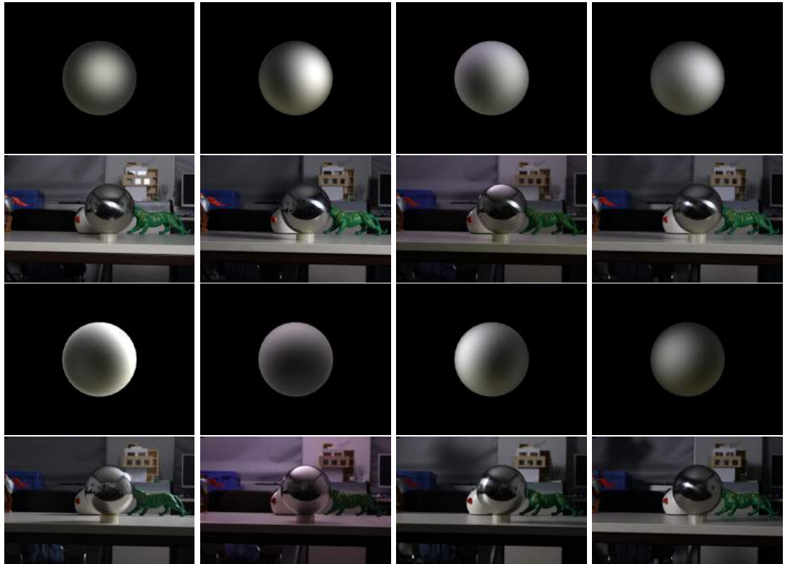
Figure 4.7: The eight light ground truth lighting conditions. The renderings in the black boxes show the reconstructed ground truth lighting functions. The image below each of them shows one of the images which were used to create the HDR image.
