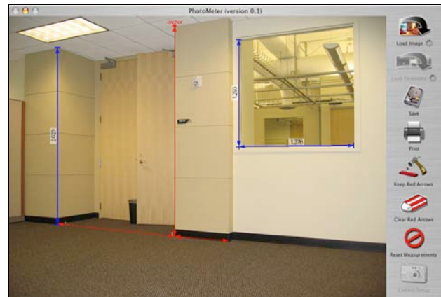
Figure 6: The user interface of PhotoMeter. This screenshot also shows measurements that are already saved (blue arrows with dimensions) and a measurement series that is still in progress (red arrows with anchor).
