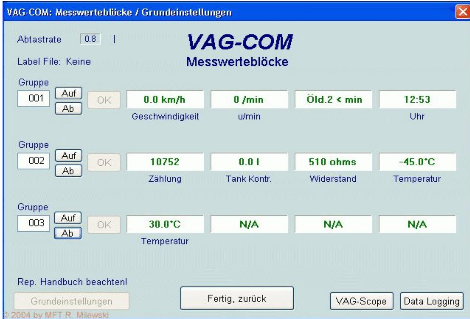
The screenshot shows the VAG-COM software interface for reading sensor values. The window title is "VAG-COM: Messwerteblocke / Grundeinstellungen". The interface displays three groups of sensor data, each with a group number, a set of control buttons, and four data fields with their respective units.
