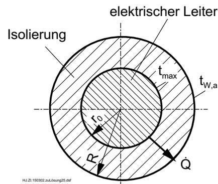
$$\dot{Q} = I_{max}^2 R_{\Omega} = \frac{t_{max} - t_{W,a}}{R_{\lambda,Is}}$$
