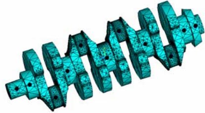
Figure 4 Elastic Crankshaft – FEM discretized – master nodes as black points
