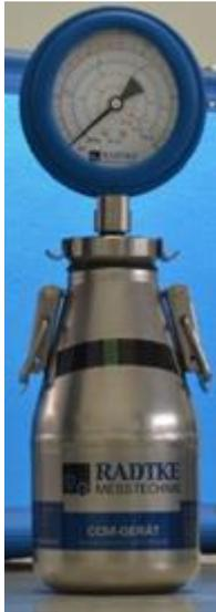
Fig. 22 CM measuring device for humidity measurement (radtke-messtechnik.com)
