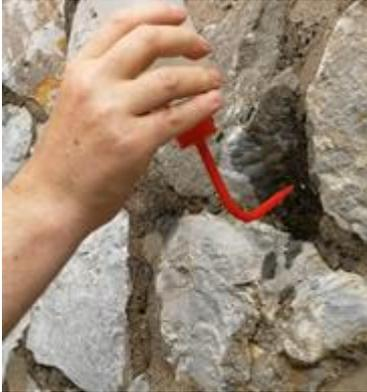
Fig. 23 Wetting test on a natural stone façade
