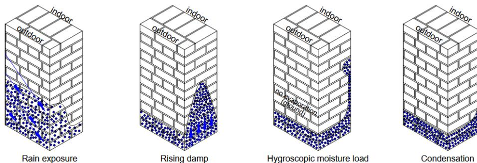
Fig. 4 Schematic representation of moisture distribution in masonry
