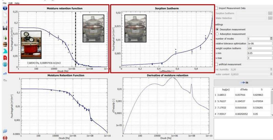
Figure 3: Screenshot of the MaterialGenerator: Fitting of the moisture retention curve with the help of desorption values and values of overhygroscopic water content
