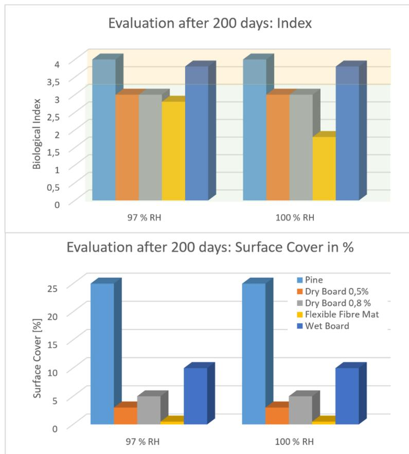
Figure 27: Evaluation of biological processes according to Table 4 after 200 days (top) and coverage of the specimen surface with decay mycelium in percent (bottom) at the boxes with initially 97 % RH (left) and 100 % RH (right).
