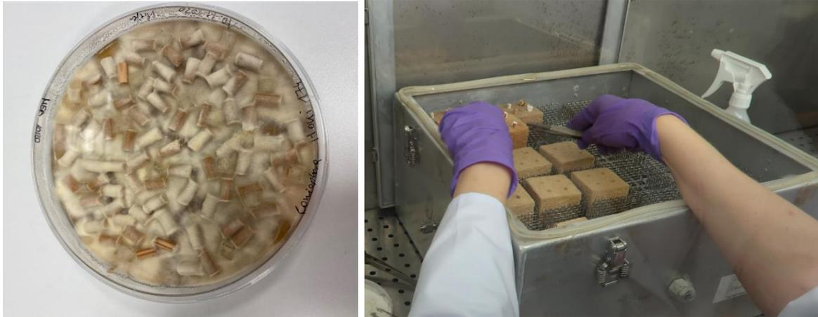
Figure 16: Overgrown wooden dowels with test fungi *Coniophora Puteana* (left) and transfer of the dowels into the test specimen (right).
