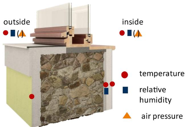
Figure 40: Position of the sensors for an interior insulation measuring section
