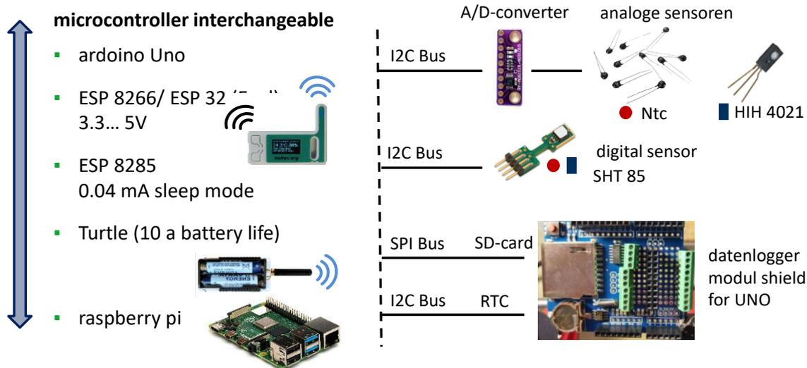
Figure 41: Commercially available board/microcontroller and sensors connected via bus system
