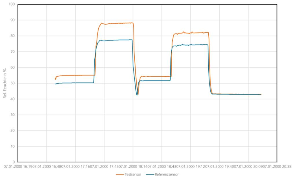
Figure 48: Calibration measurement of the used HIH sensor in comparison with the reference sensor
