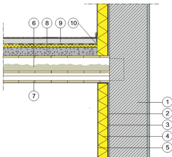
Figure 39: Detailed drawing for the insulation of a joist support in case it is not possible to open the ceiling between two floors
