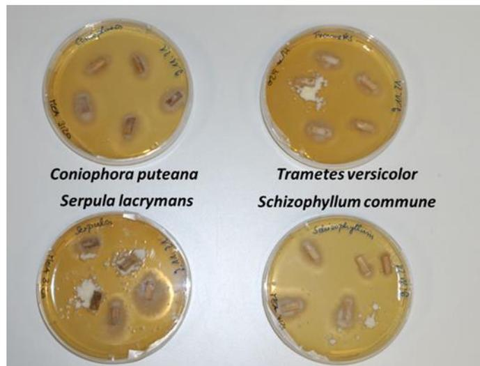
Figure 31: Re-inoculated dowels from the specimens at the end of the lab test investigations.
