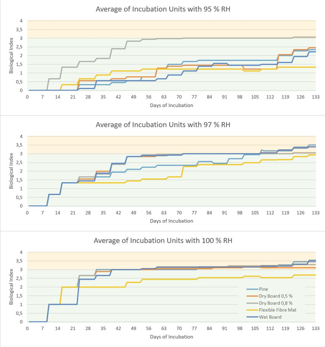
Figure 26: Evaluation of biological processes according to Table 4 during the first 133 days: Different growths speed on the dowels of the 4 test materials and the reference specimens. Only Pine and the wet board reach values up to 3.5 in that period.
