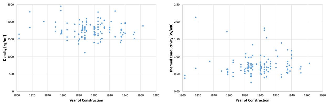
Figure 8: Density and thermal conductivity of 200 test specimens measured in the laboratory of the IBK
