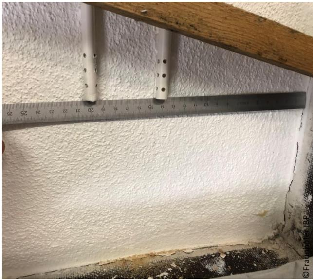
Figure 52: Perforated plastic tubes for the installation of the temperature and rel. humidity sensors within the interior insulation system
