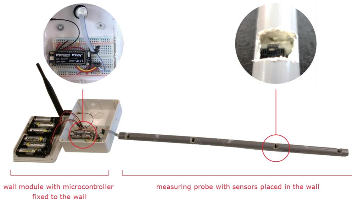
Figure 58: Overview of the measurement node
