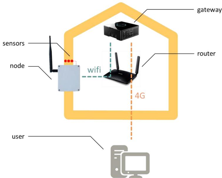
Figure 61: Principle of data transmission using the WiFi configuration
