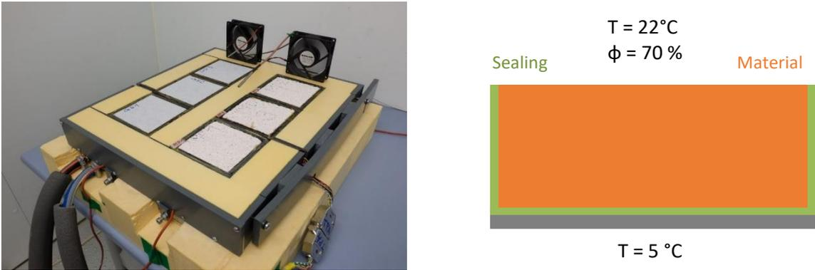
Figure 33: Left: schematic structure of the condensation test, right: boundary conditions during the test
