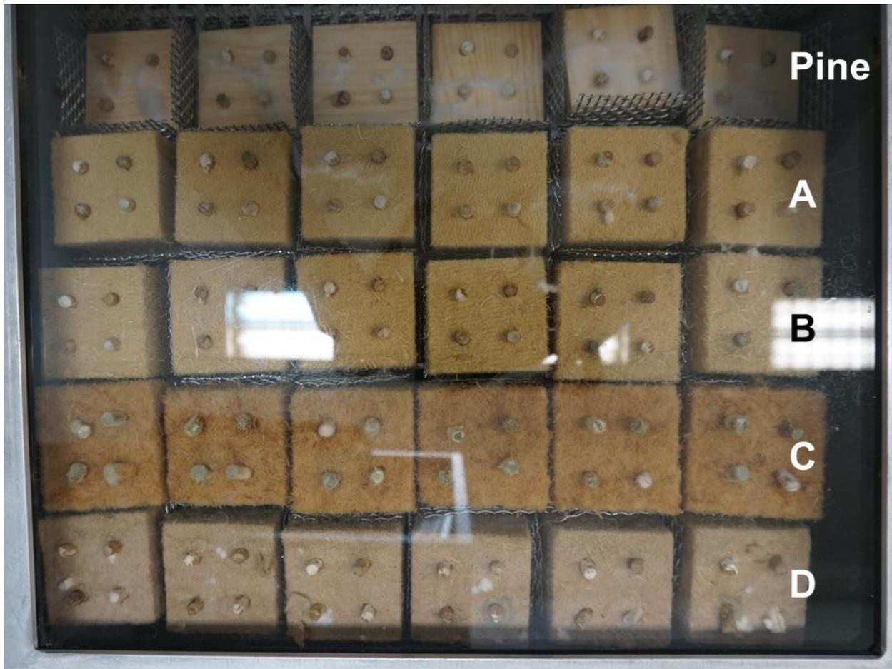
Figure 18: Visual observation after 25 weeks: Some mould growth appeared in two of the 6 incubation units. It was initially observed on the dowels of the flexible fibre insulation C after 12 weeks.
