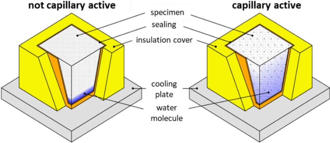
Figure 32: Schematic moisture distribution in two interior insulation materials without liquid transport (left) and with significant liquid transport (right) during the Kapitest.
