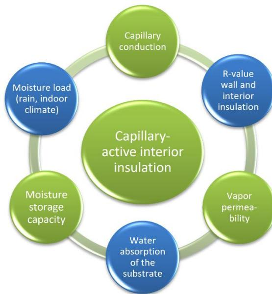
Figure 37: Development Influencing factors for the moisture performance of capillary-active insulation materials. The green factors are parameters of the insulation system, the blue ones factors of the boundaries and the substrate wall. By application limits the blue factors are eliminated to be able to focus on the insulation system itself.
