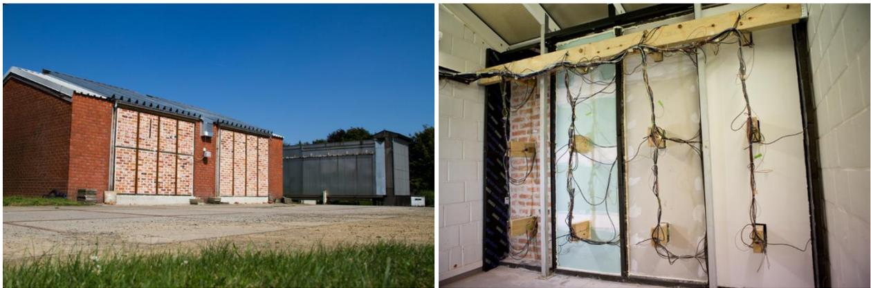
Figure 38: Left: Test house at the BBRI test facility; right: One of the two test chambers at the BBRI test facility from the inside. From left to right: non-insulated wall, EPS, mineral wool and calcium silicate. The three beams per wall represent a different connection between masonry and beam. The top beam parallel to the wall only serves as a structural support for the wall
