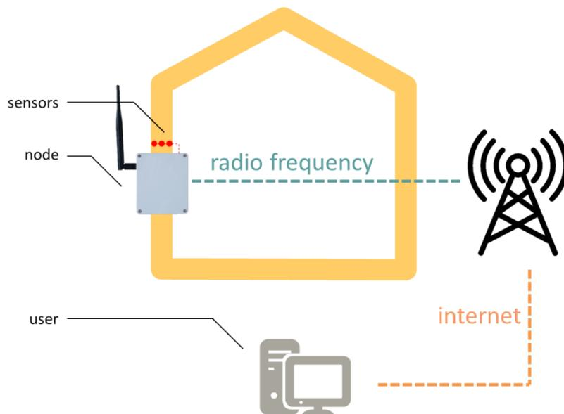
Figure 63: Principle of data transmission using the Sigfox configuration
