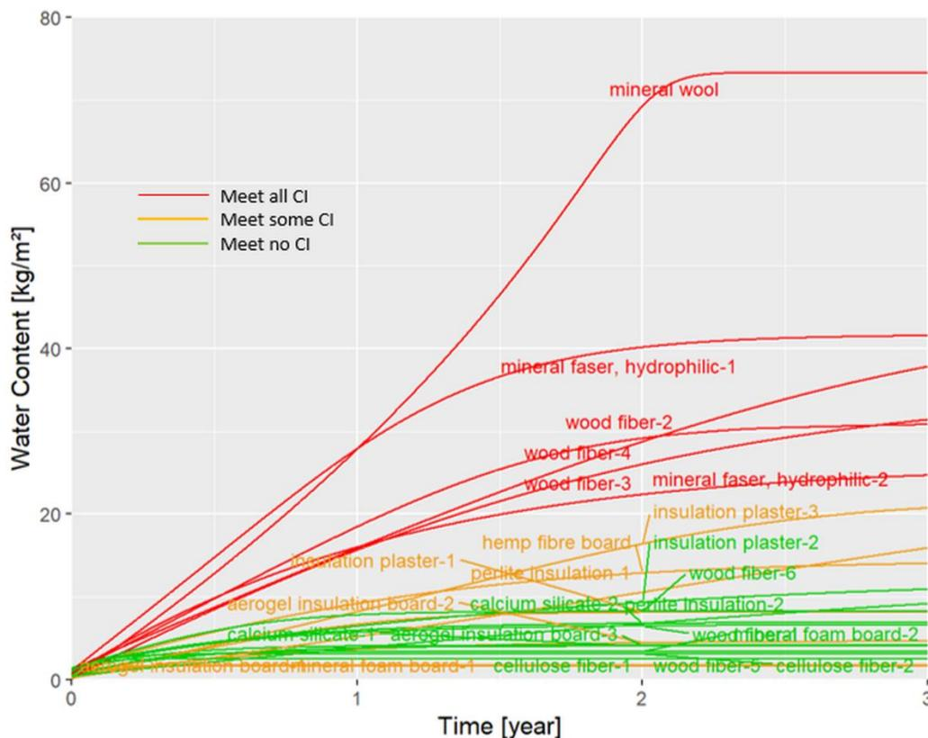
Figure 34: Development of the water content in the interior insulation material over three years. Contraindicator (CI): significant and continuous increase of total water content.
