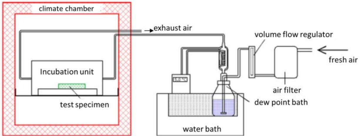
Figure 17: Test setup for the incubation period in the lab with climate chamber at 25 °C, incubation unit and supply of preconditioned and filtered air.
