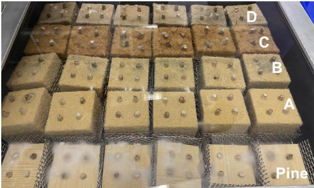
Figure 23: Visual observation after 40 weeks: Clearly strongest mycelium growth on the Pine, mould growth on materials B and D as well as on the dowels of material C. Some visible growth of mould and decay fungi on material A.
