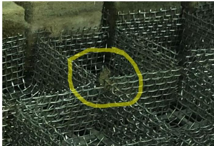
Figure 28: Parts of the flexible fibre mat stuck to the metal basket.
