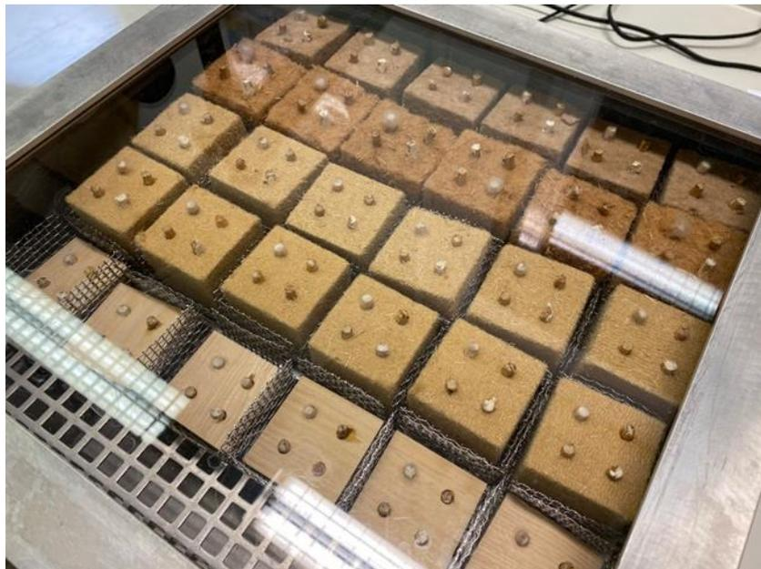
Figure 19: Test specimens with overgrown dowels in an incubation unit. View through the glazed lid.
