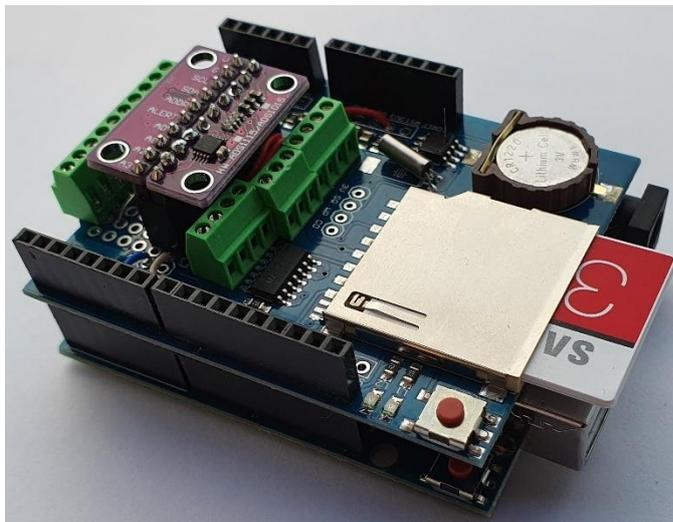
Figure 42: Prototype setup consisting of an Arduino UNO R3 with a data logger-module (SD card with RTC real time clock), 5 x NTC, 1 x HIH 4021 and 5 x I2C bus (2 x AD converter)
