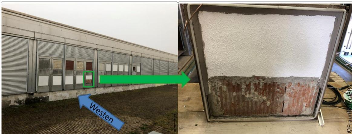
Figure 51: Installation situation of the measurement system in the outdoor test facility at the Holzkirchen site. Left: the test specimen in its installed state. Right: the figure shows the surface design of the test specimen with the exterior plaster removed
