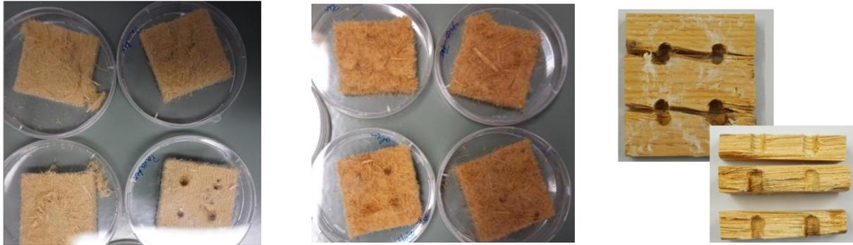
Figure 30: Cut specimens after 40 weeks of incubation. Dry board A (left), flexible mat C (middle) were horizontal sliced and pine sapwood (right) was cut along holes,
