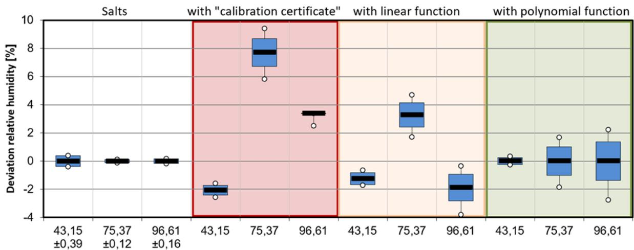
Figure 50: Accuracy data for the HIH humidity sensor using desiccators with 3 humidity levels
