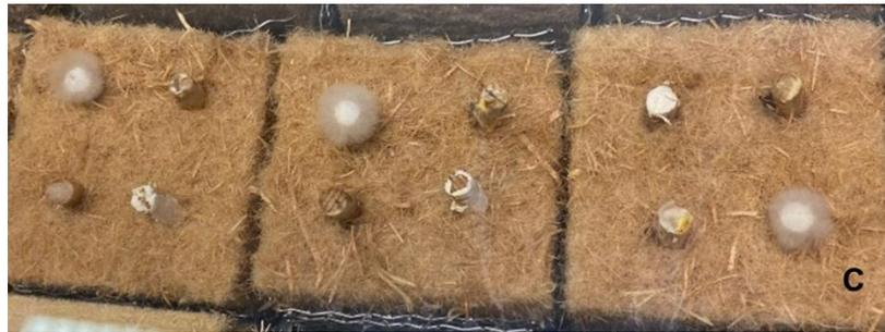
Figure 20: Visual observation after 8 weeks: fungi growth on the dowels in the flexible fibre insulation C. While a strong mycelium growth of *Schizophyllum commune* can be detected on the dowel itself (but no transfer to the specimen) only moderate growth can occur for the three other fungi.
