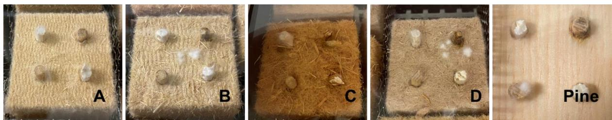
Figure 21: Visual observation after 8 weeks: established mycelium growth on all specimens apart from the flexible fibre mat C
