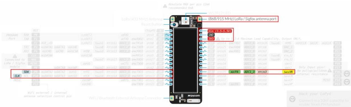
Figure 59: Pycom LoPy4 pinout with the pins used in the prototype indicated in red
