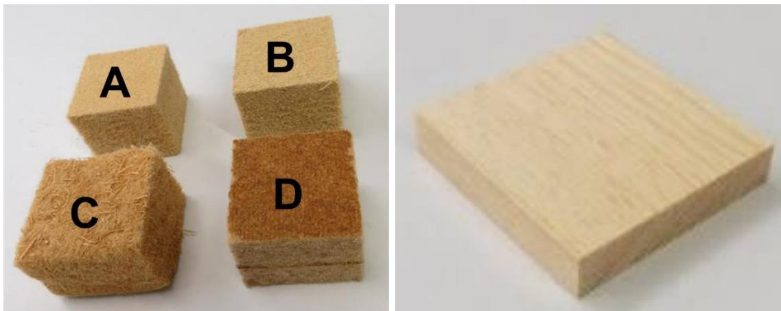
Figure 15: The four investigated wood fibre insulation materials A, B, C, D described in Table 2 (left) and the reference material solid Pine sapwood (right)
