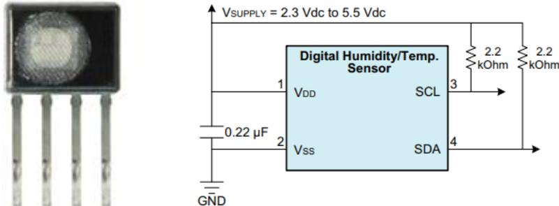
Figure 56: Honeywell HIH 8121 sensor and its typical application circuit (source: Honeywell)
