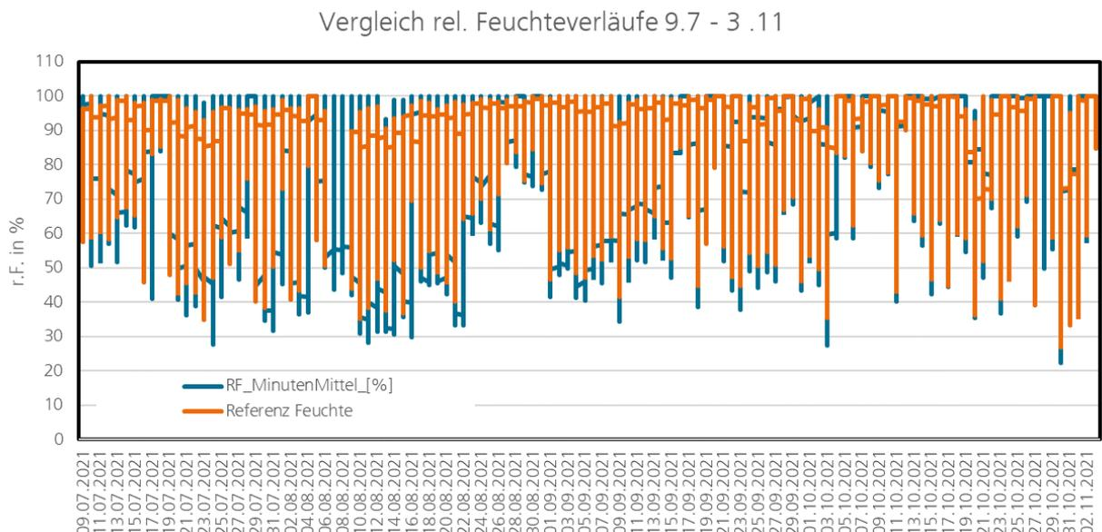
Figure 55: Comparison of the relative humidity between the newly invented measurement system and the reference measurement at the meteorological station.
