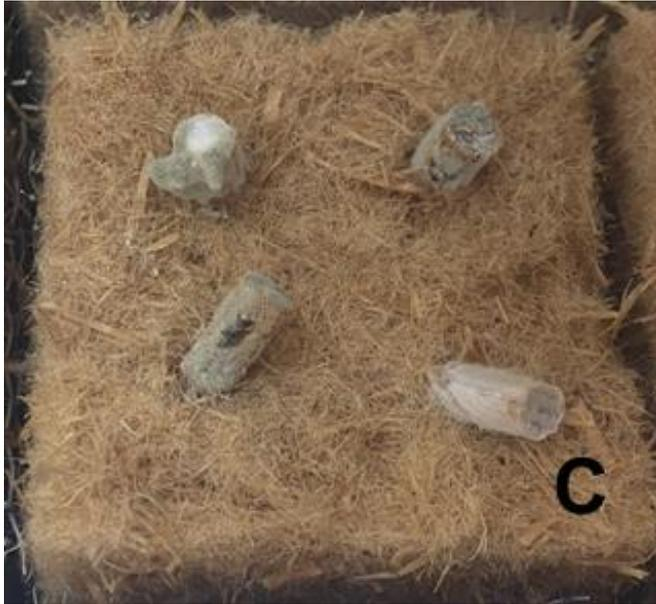
Figure 24: Visual observation after 40 weeks: Mould growth on the dowels of the flexible fibre mat C but not on the specimen.
