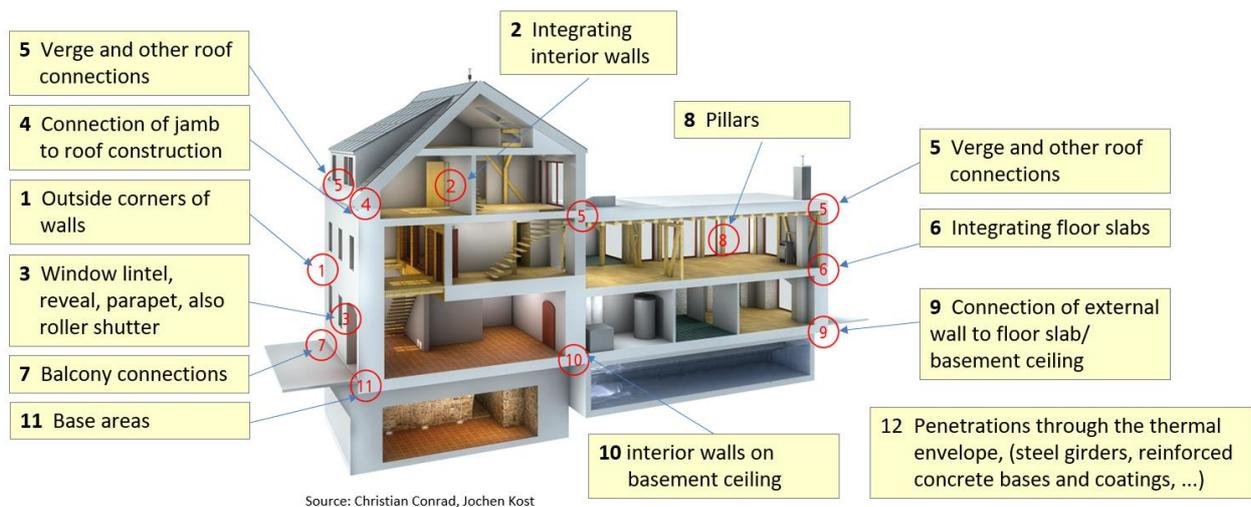
Figure 14: Illustration of common critical connection details in buildings with internal insulation
