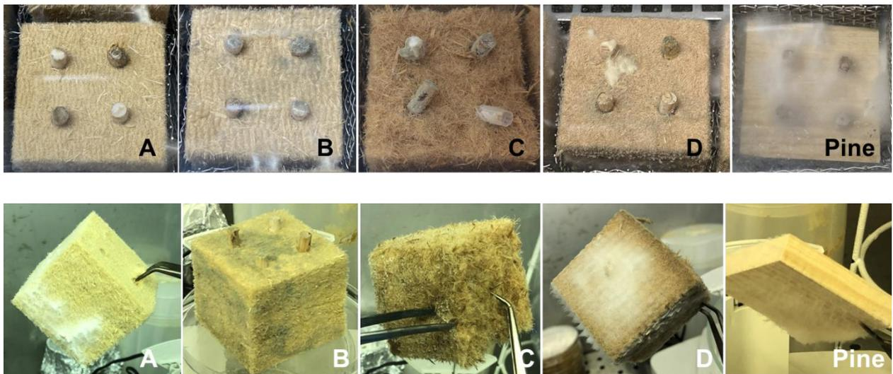
Figure 25: Visual observation after 48 weeks: View from the top (top) and from the bottom or side (bottom). Strongest growth of decay fungi mycelium on the pine specimen, but present also on all other specimens.
