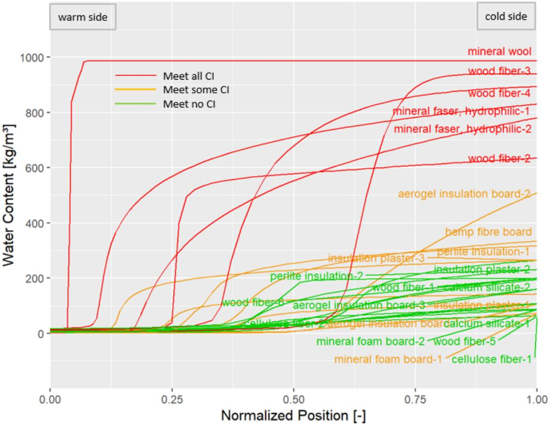
Figure 35: Water content profiles over the normalized thickness after three years of simulation. Contraindicator (CI): high absolute water content on the cold side.
