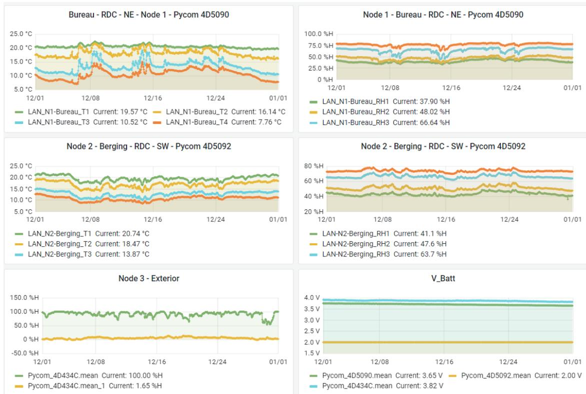
Figure 64: Example of data visualisation in Grafana. Two nodes measure temperature and relative humidity inside the wall, a third one measures the outside conditions. Battery voltage of these three nodes is also visualised.
