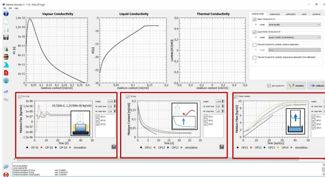
Figure 4: Screenshot of the MaterialGenerator: Calibration of moisture transport function (vapour and liquid water) with the help of results from drying experiment, water uptake experiment and dry cup experiment
