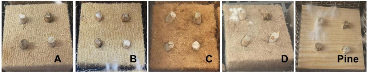
Figure 22: Visual observation after 23 weeks: Strongest decay mycelium growth on the Pine, followed by the “wet” board D and the “dry” boards B and A. C still shows no growth at all – also the mycelium on the dowel disappeared.
