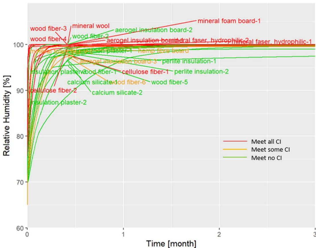
Figure 36: Development of the Relative Humidity in the pores of the insulation material at the vapor tight, cold side of the insulation layer. Contraindicator (CI): RH reaches 100 % on the cold side rather quickly.
