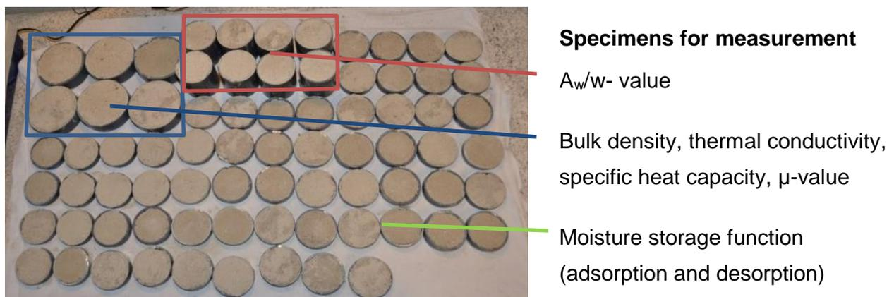
Figure 2: Specimens for the determination of hygrothermal material properties
