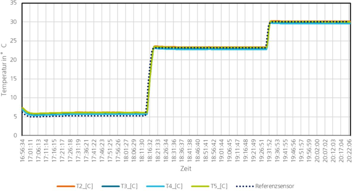
Figure 45: Calibration measurement of the used NTC's in comparison with the reference sensor.
