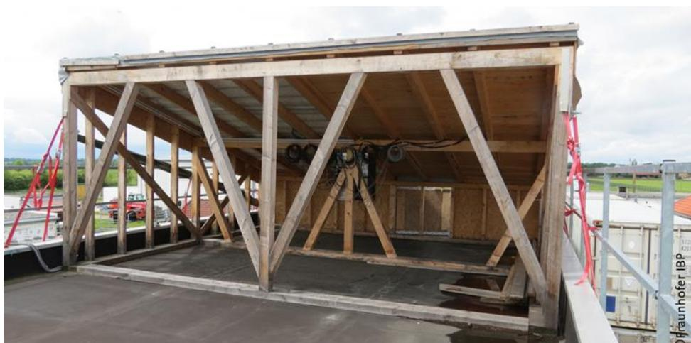
Figure 53: Flat roof test bench within the field test facility at the Fraunhofer IBP in Holzkirchen
