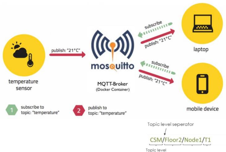
Figure 62: General principle of a MQTT server
