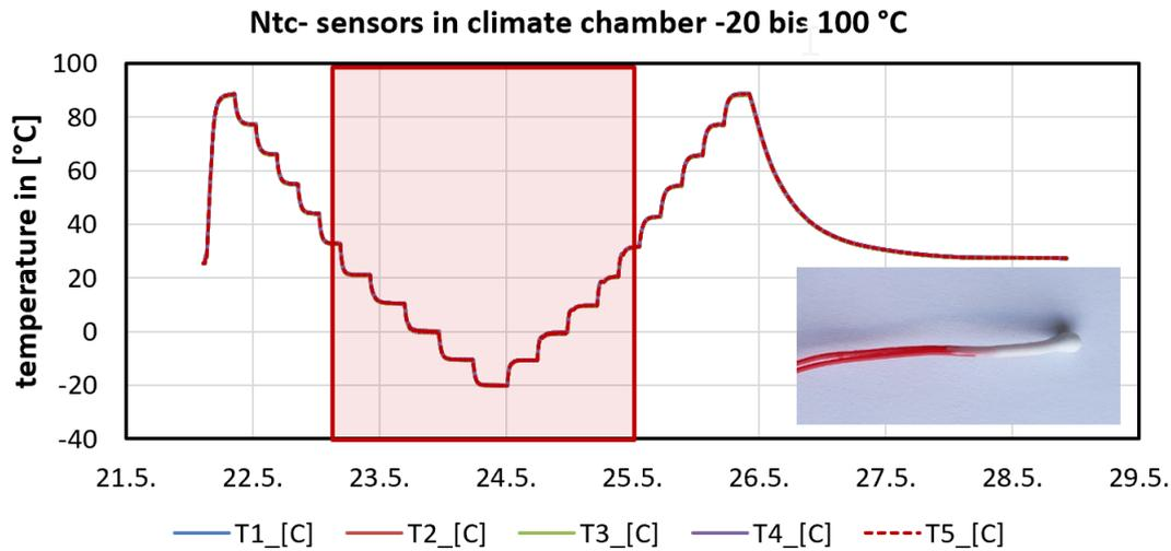
Figure 46: Testing in the climatic chamber, NTC with liquid plastic
