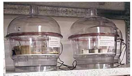
Figure 49: Calibration by means of desiccator with 3 humidity levels
