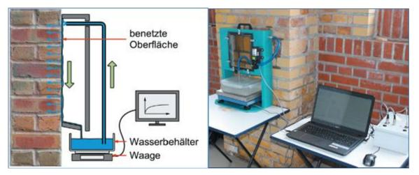
Fig. 26 Water absorption measuring device, measuring principle and practical application [hf-sensor.de]
