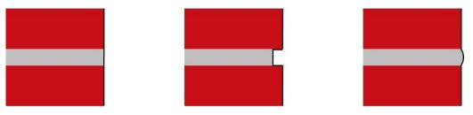
Fig. 15 Typical form of mortar joints: left: flush with the wall, middle; a shadow joints, right: a beaded joint
