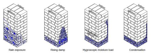
Fig. 4 Schematic representation of moisture distribution in masonry
