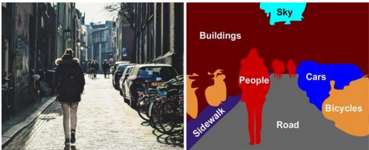
Figure 16 Example of semantic segmentation (Géron, 2023, p. 492)
