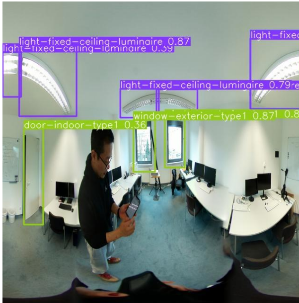
Figure 77 Sample image from batch 0 in the test run. The radiators below the windows were not recognized. Image from (Bendiek Laranjo, 2023)
