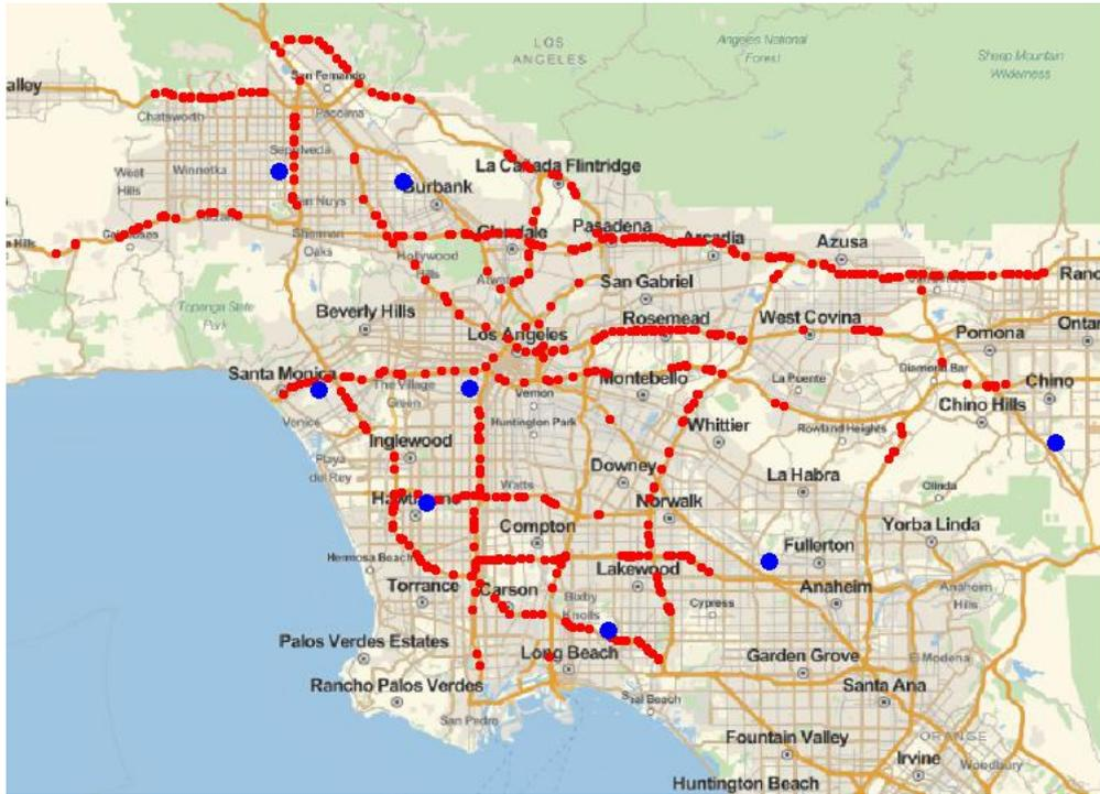
**Figure 4.5:** Map of the Los Angeles Metro Area. Small red dots represent traffic sensors, while large blue dots represent Weather Stations. No suitable Weather Station exists around the Rosemead area.
