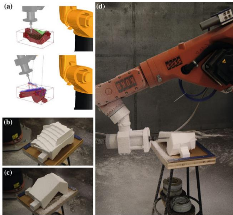
Figure 2.4 Robotic milling for one rib segment (Jung et al. 2016)
