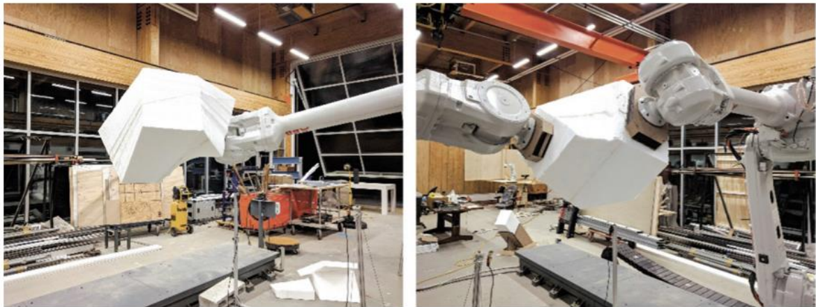
Figure 2.10 fabrication process of element for the connections of branches (Wu and Kilian 2020)
