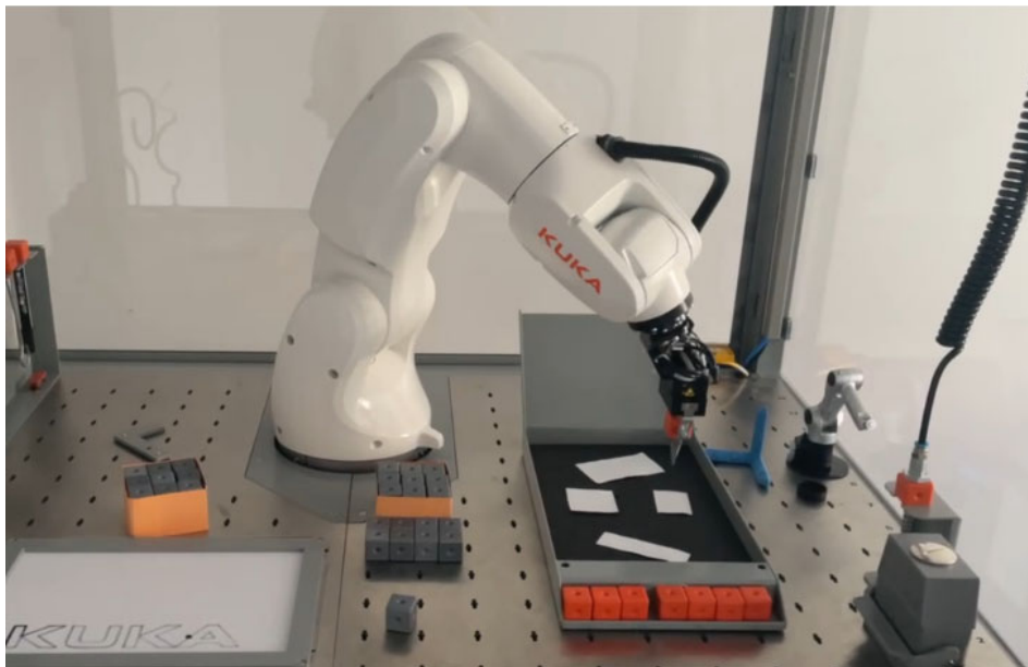
Fig 34 The robotic arm, guided by the vision program, moves to the irregular object's placement location.
