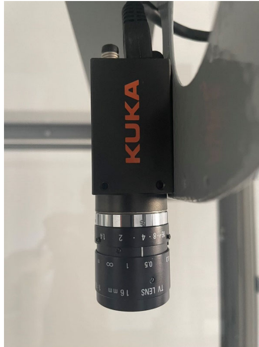
Fig 28 VCXG-25M industrial camera
