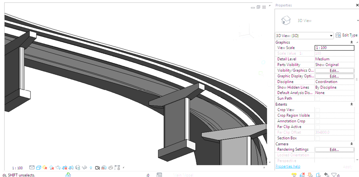
Fig. 35 Bridge for the case №1 generated in Dynamo and exported in Revit project file.
