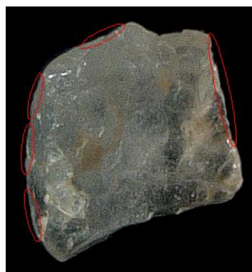
Fig. 3: Determination of the irregularity of a grain from w7 sand (220 pixels/mm resolution)
