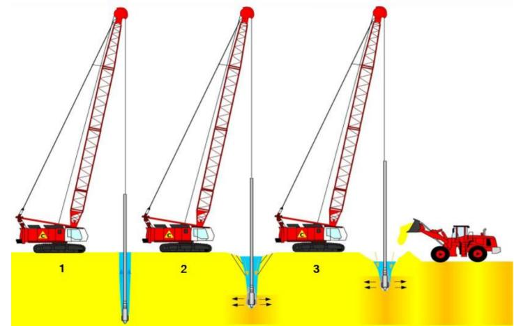
Fig. 2: Cross section and operating mode of the depth vibrator; adapted from Keller (2019) and Kirsch (2017)
