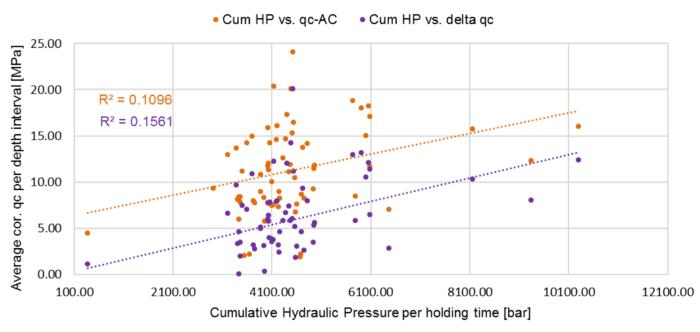
Fig. 5: Correlation between cumulative hydraulic pressure and after compaction (orange) or  $\Delta q_c$  (purple).
