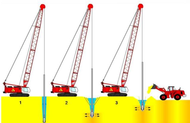
Fig. 1: Vibro compaction procedure; Cofra (2019)
