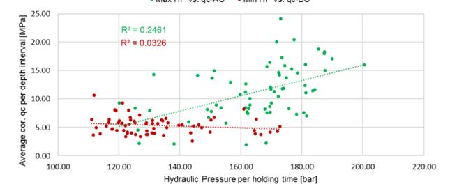
Fig. 4: Correlation between minimum hydraulic pressure and before compaction  $q_c$  (red) and correlation between maximum hydraulic pressure and after compaction  $q_c$  (green).
