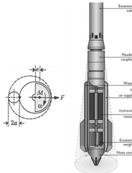
Fig. 2: Cross section and operating mode of the depth vibrator; adapted from Keller (2019) and Kirsch (2017)
