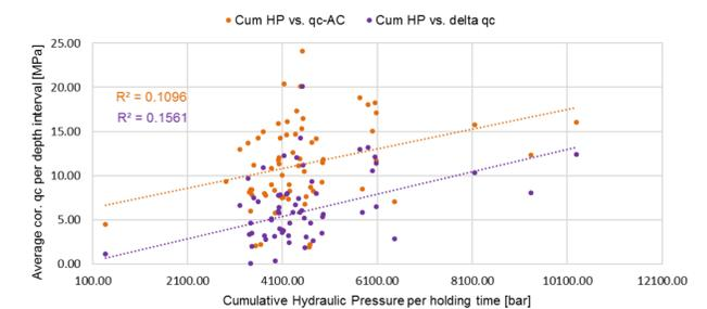
Fig. 5: Correlation between cumulative hydraulic pressure and after compaction (orange) or  $\Delta q_c$  (purple).
