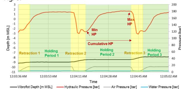
Fig. 3: Typical time history of the vibrator depth, hydraulic pressure, air pressure and water pressure during holding and retraction
