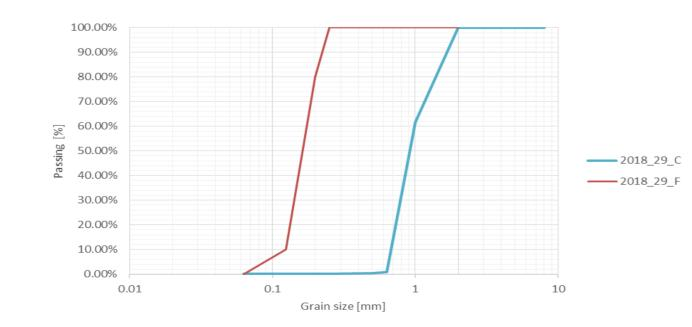
Fig. 1: Grain size distribution curves of coarse (2018\_29\_C) and fine sand (2018\_29\_F).
