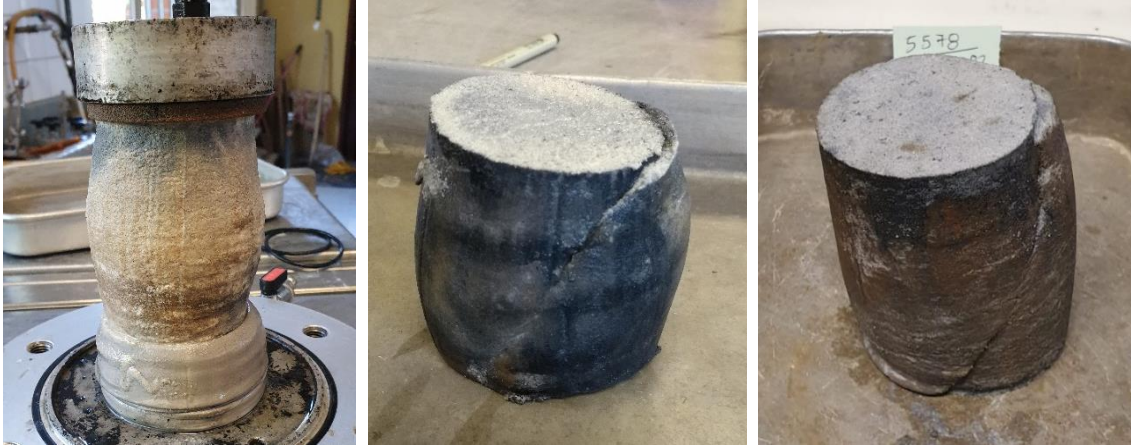
Figure 3.9: Specimen appearance after shearing (left 50 kPa, middle 280 kPa; left 500kPa)
