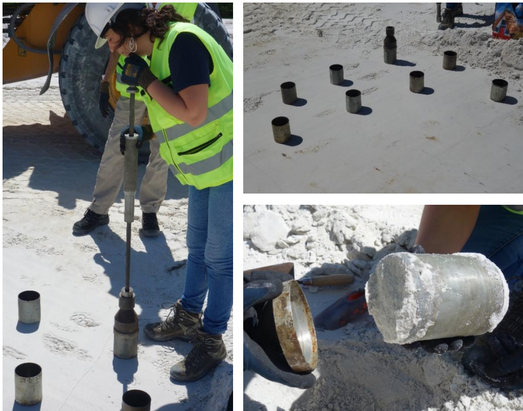
Figure 1.6: Procedure of sampling by cylindrical cutter. (a) distribution of cylinder on the soil's surface, (b) driving by impact, (c) excavation and sealing
