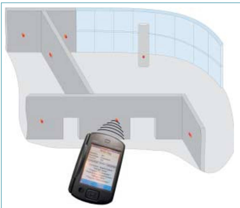
Fig. 3 "Smart elements" – labeling of elements by means of transponders.
