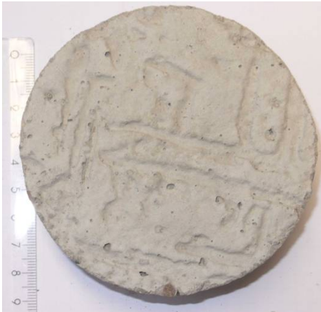
Figure 3. Specimen prepared with form liner.
