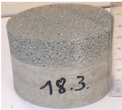
Figure 4. Specimen prepared with sound absorbing silica sand coating.
