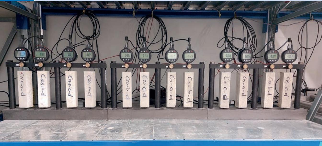
Ausdehnungstests an Betonproben | Expansion test on concrete samples | Photo: Mohammed K. Dahir
