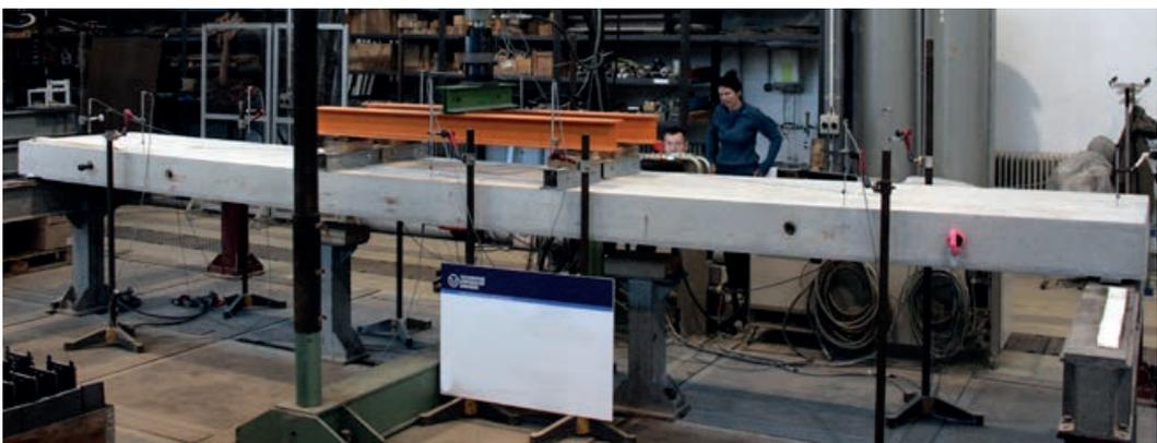
Determination of the flexural resistance of a strengthened reinforced concrete slab | Photo: Frank Schloditz
