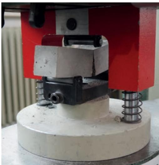
Biegezugversuch an einem Feinbetonprisma | Bending tensile test on a fine-grained concrete prism | Photo: Karoline Holz
