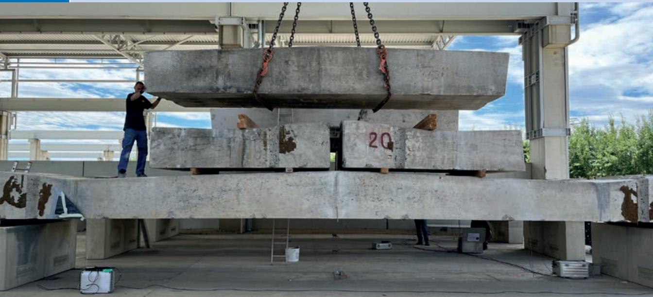
Vorversuche an alten Brückenträgern – Installation der Dauerbelastung | Preliminary tests on old bridge girders – installation of long term loading | Photo: Max Herbers
