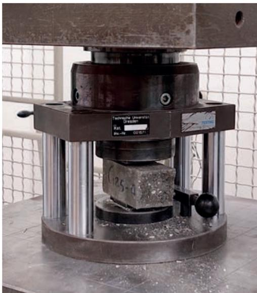
Druckversuch an Feinbeton | *Compression test on fine grained concrete* | Photo: Mohammed K. Dahir
