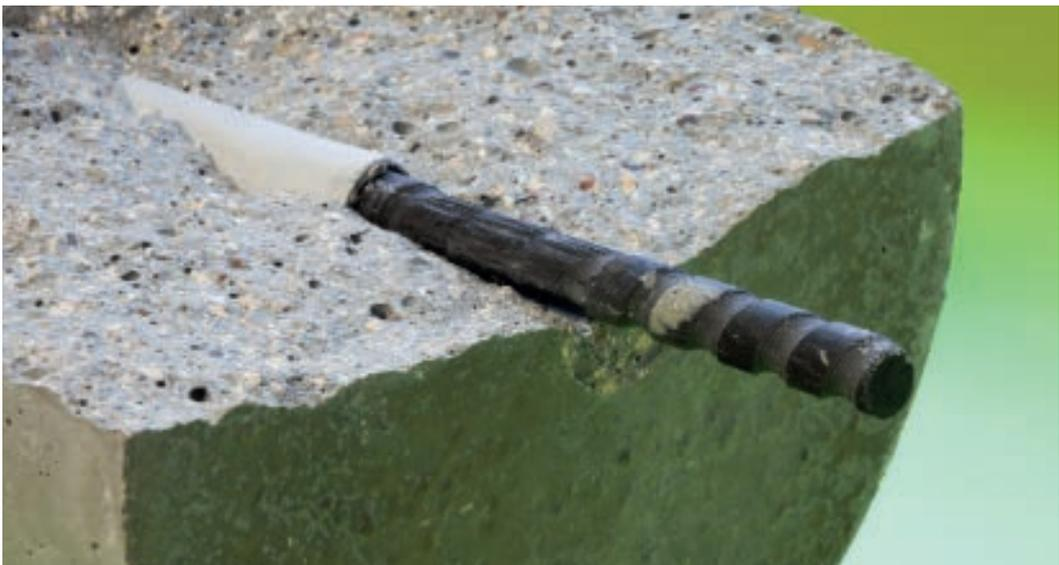
Carbon fiber reinforcement bar in concrete | Photo: Sven Hofmann
