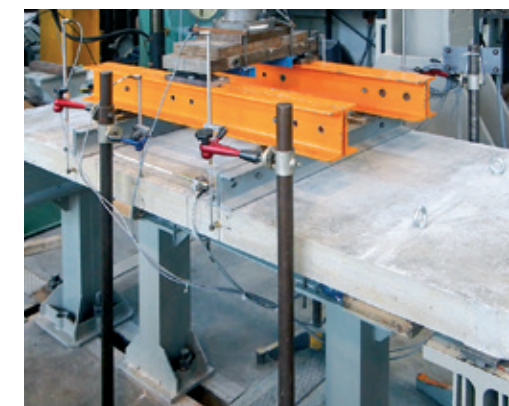
4-Punkt-Biegeversuch am Deckenelement | 4-point bending test of the ceiling | Photo: Alexander Schumann
