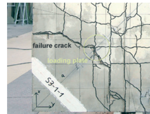
Typisches Rissbild in einem Quadranten, Plattenunterseite | Typical crack formation in a quarter of a tested slab, view of the bottom side | Photo: Michael Frenzel
