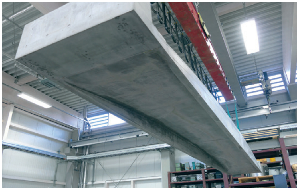
Unteransicht des leichten Deckenelementes aus Carbonbeton | Bottom view of the light ceiling element made of carbon reinforced concrete | Photo: Sebastian May
