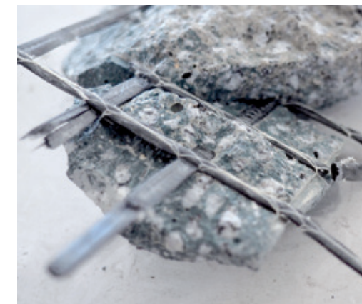
Carbonbewehrtes Abbruchmaterial | Carbon reinforced demolition material | Photo: Sebastian May
