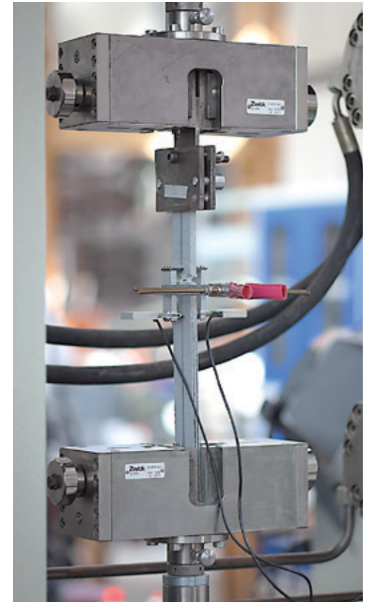
Auszugversuch an Carbonbeton | Pull-out test on a carbon concrete specimen | Photo: Ulrich van Stipriaan
