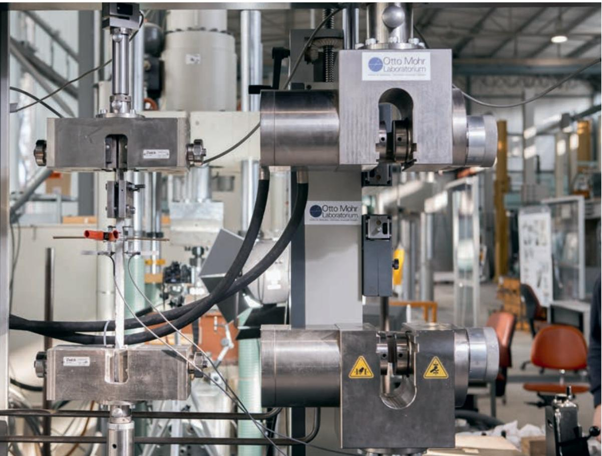
Zug-Druckprüfmaschine (Typ Zwick) | Tension-compression testing machine (type Zwick) | Photo: Jörg Singer
