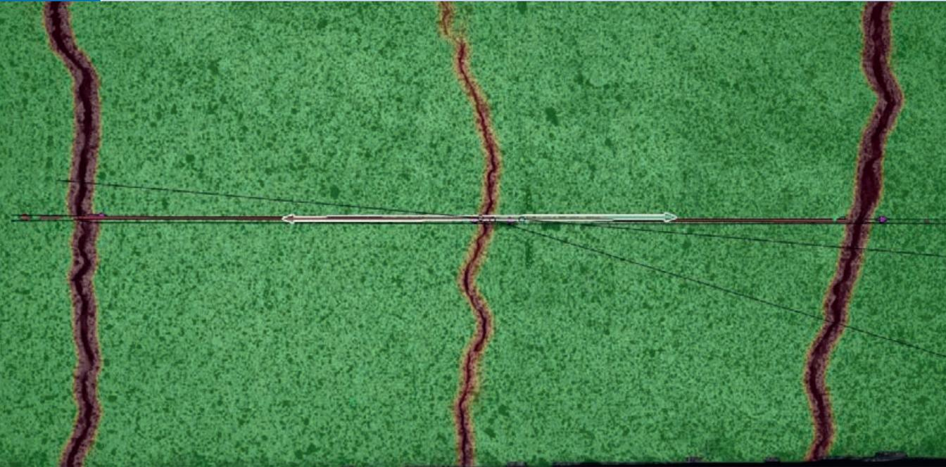
Photogrammetrische Messung der Risse im Carbonbeton in ARAMIS® | Photogrammetric measurement of cracks in carbon concrete in ARAMIS® | Graphic: Sandra Zögermann, Kristina Farwig
