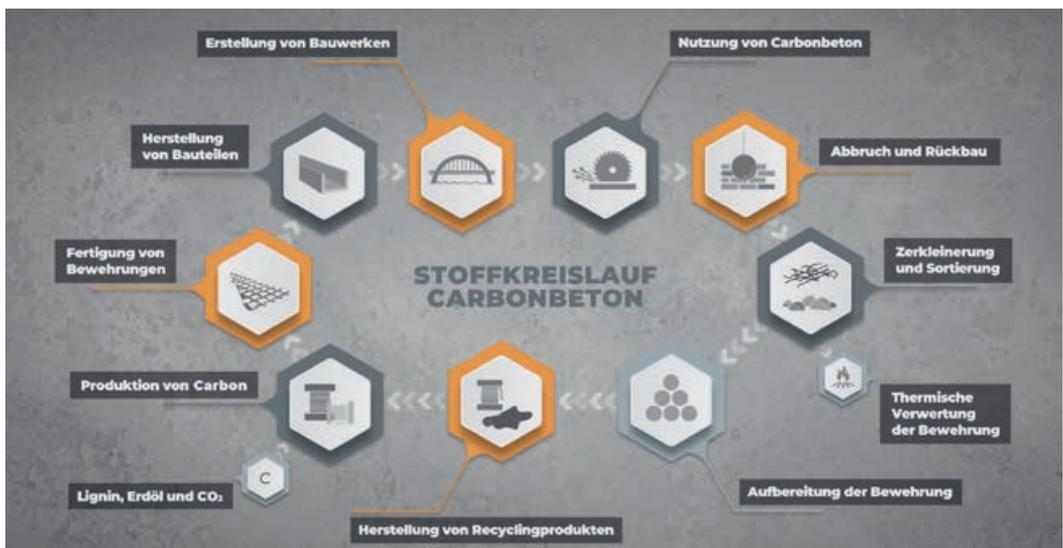
Der geschlossene Stoffkreislauf von Carbonbeton | The closed material cycle of carbon reinforced concrete | Graphic: filmaton
