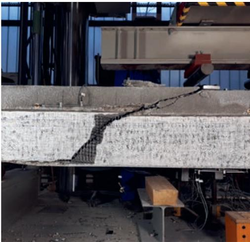
Biegeschubversagen eines Plattenbalkens | *Shear failure of a T-beam* | Photo: Sebastian May
