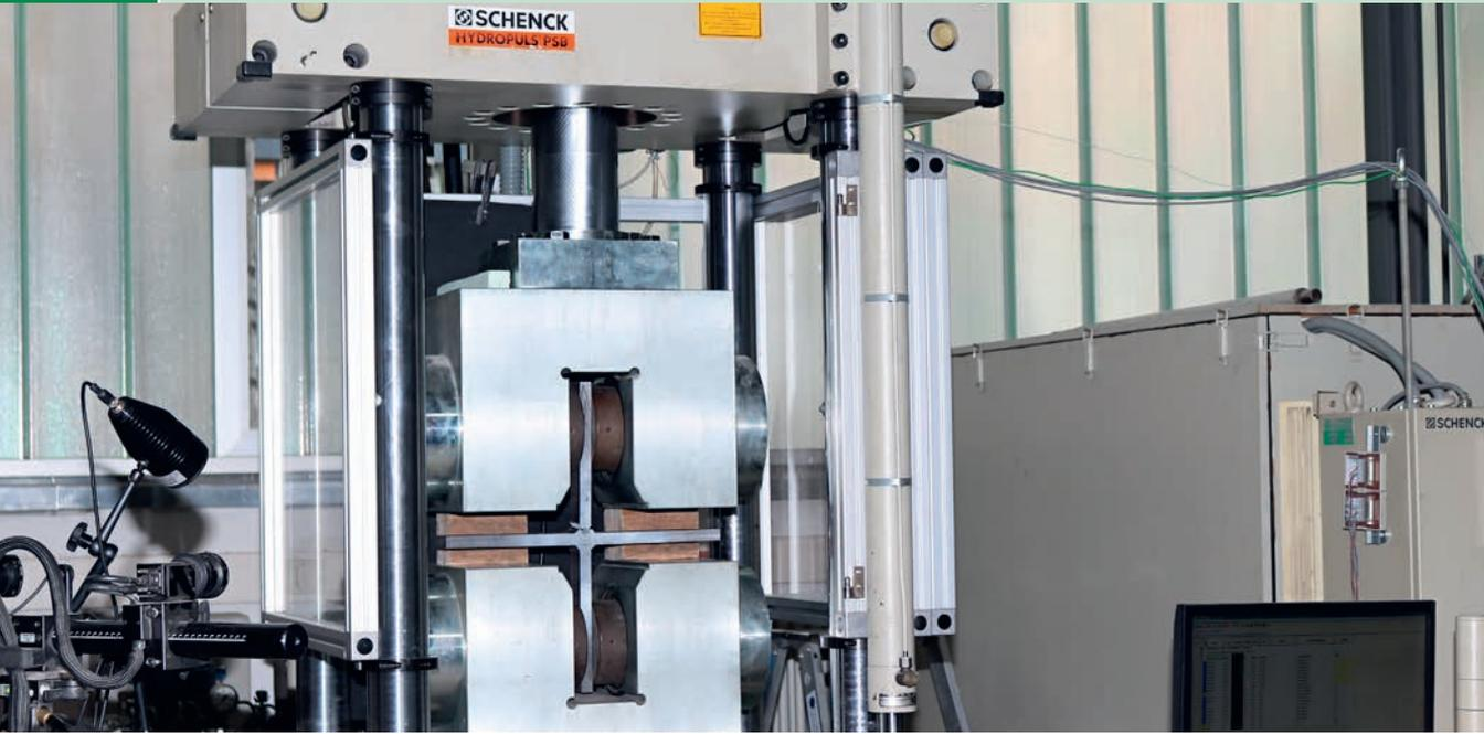
Prüfmaschine Schenck 1000 kN | Universal testing machine Schenck 1,000 kN | Photo: Thomas Häntzschel
