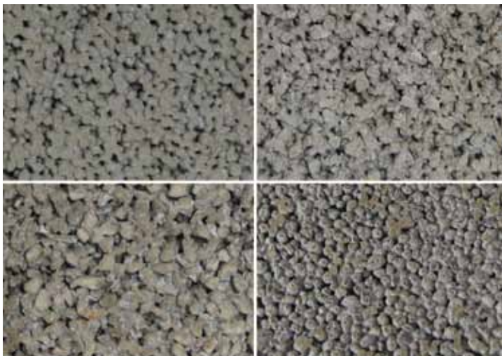
Oberflächen haufwerksporiger Leichtbetone Surfaces of lightweight aggregate concrete with open structure
