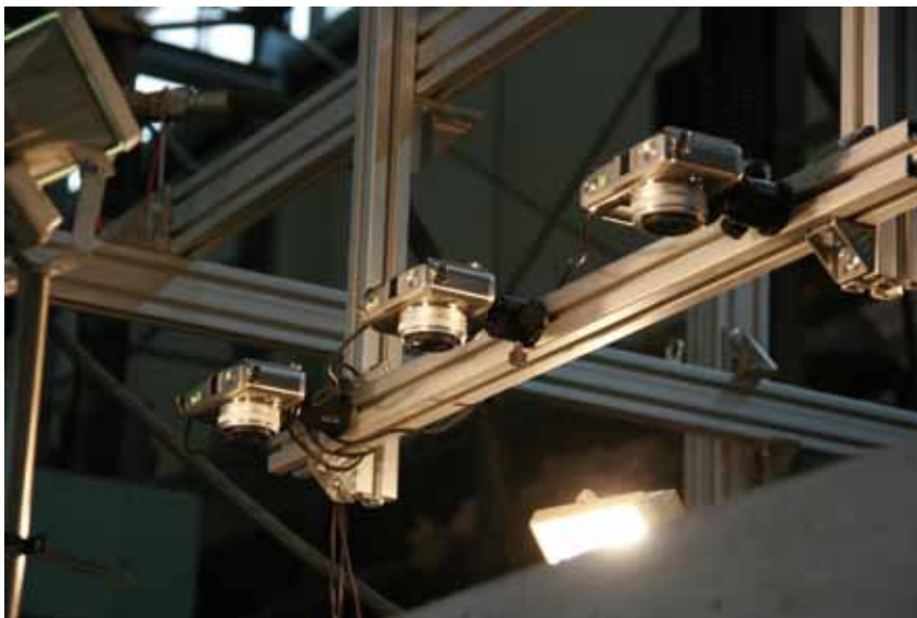
Angepasste 2D-Photogrammetrie- anlage Adapted Reinforcement 2D photogrammetry system
