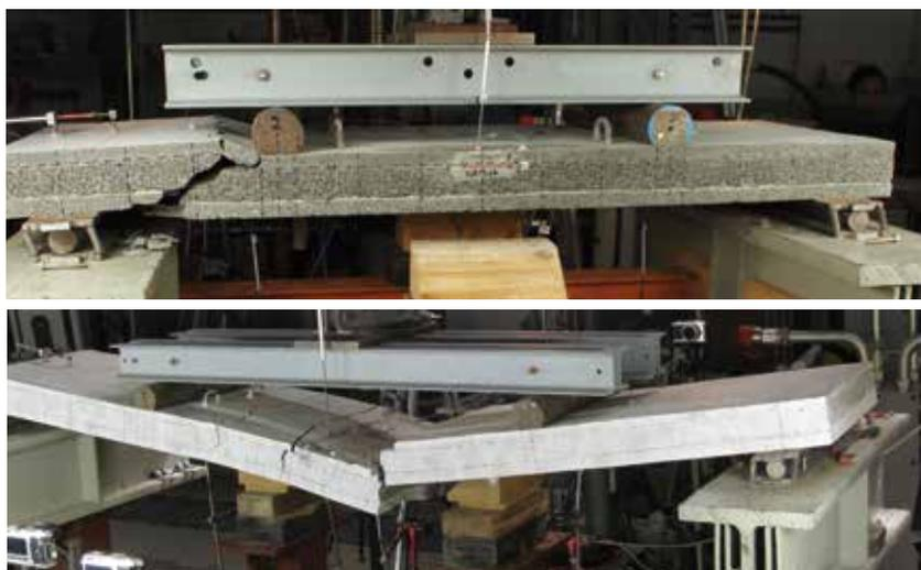
Schubversagen (oben) | *Shear failure (top)*.
