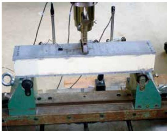
*Bending test on textile reinforced concrete sandwich elements. Photo: Cosmin Balaj*
