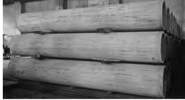
Figure 38 Precast prestressed pipes for the Oued-Fodda project
