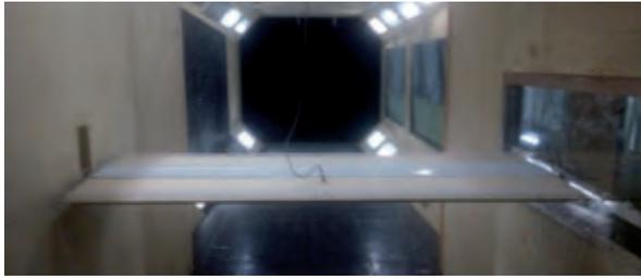
Fig. 13 Sectional model test in a wind channel
