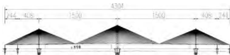
Fig. 11 Span arrangement of Qiongzhou Strait Cable-Stayed Bridge
