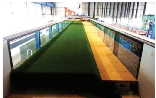
Figure 4. Model set up with half a trapezoidal compound open—channel.
