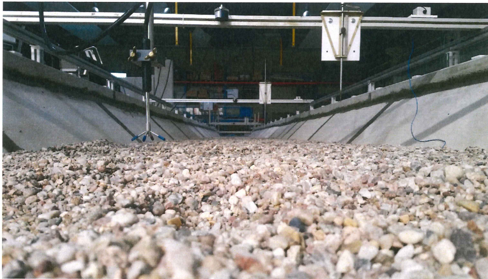
Figure 8. Impression of the experimental flume with bare concrete slopes.
