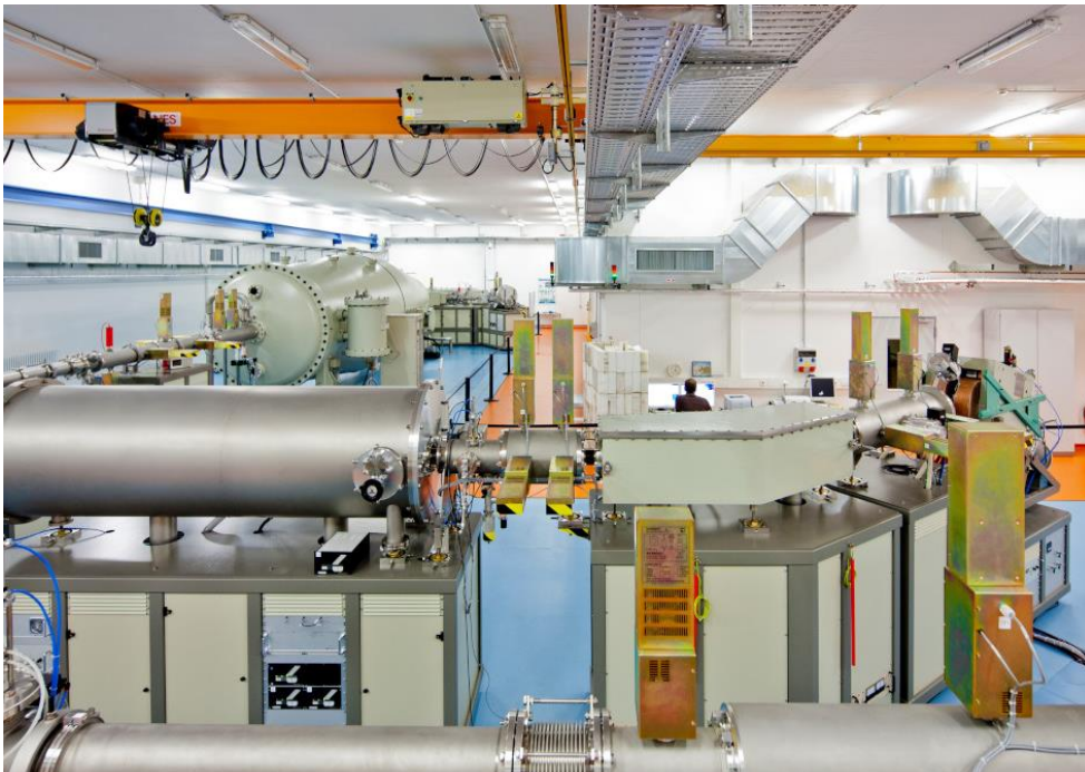
Fig 1: 6 MV tandemron DREAMS at Helmholtz-Zentrum Dresden-Rossendorf used for AMS analysis of ^{10}\text{Be} , ^{26}\text{Al} , ^{36}\text{Cl} , and other radioisotopes (©HZDR / O. Killig).
