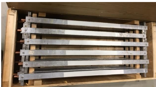
Fig.2: Copper tubes for gas-free storage of 40 mL water samples for subsequent helium extraction
