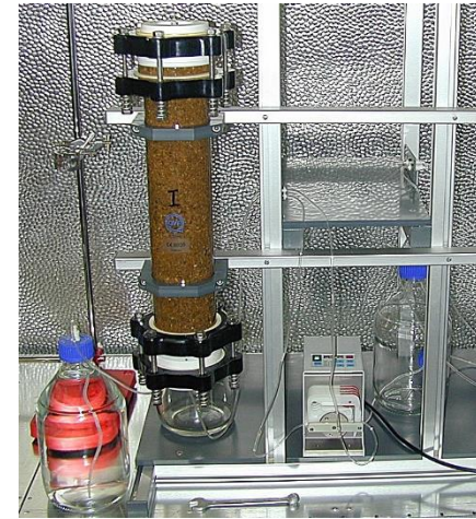
Soil column experiment setup (LfU Bayern)
