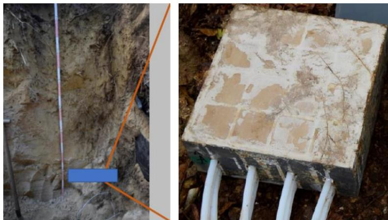
*Figure 1: Photographs of the soil profile and a segmented suction plate (16 segments). The soil was sampled above each of the 16 segments*
