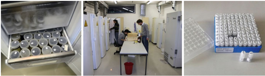
Fig. 29.5 Storage and handling of the University of Gießen Systematics and Biodiversity Collection: specimens from the Wet Collection stored permanently in 80 % ethanol in polycarbonate/polypropylene containers ( left ) in explosion-proof freezers in the underground collection room ( middle ) and DNA preps in cryotubes ( right , source: C. Albrecht)
