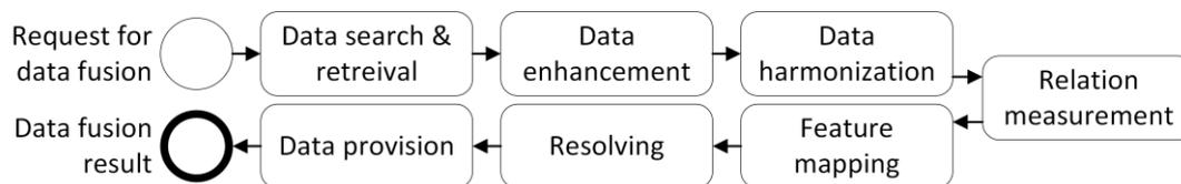
Figure 2: Low-level sub-processes for spatial data fusion.
