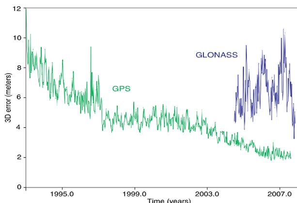
▲ **FIGURE 3** 3D-accuracy of broadcast ephemeris, based on Jet Propulsion Laboratory analysis reports (GPS) and IGS orbit combination reports (GLONASS)
