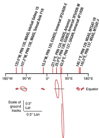
▲ FIGURE 1 SBAS satellites, their orbital positions and ground tracks (March 2008)
