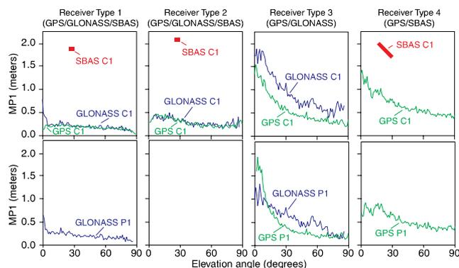
▲ **FIGURE 4** Elevation-angle-dependence of multipath and noise effects on code-phase observables for four receivers of different type
