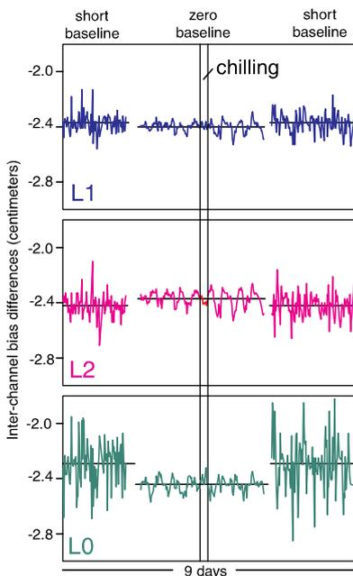
▲ FIGURE 7 Inter-channel bias differences  $c_0 \cdot \delta h^{GLONASS}$  of two receivers from different manufacturers before, during, and after a chilling experiment
