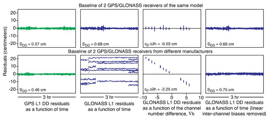
▲ FIGURE 5 Double-difference (DD) residuals on two short GPS/GLONASS baselines
