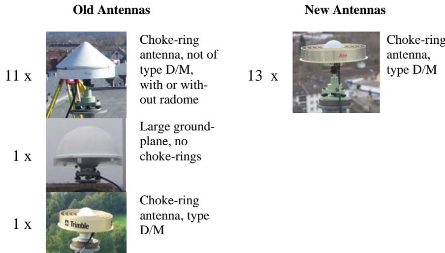
Fig. 3: Old and new antenna types
