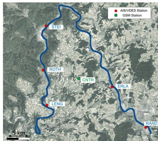
Fig. 8. Distribution of the AIS and GSM stations along the river Main.
