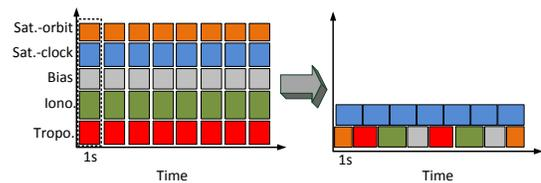
Fig. 12. Correction data reducing concept, SSR2OSR (according to [32]).
