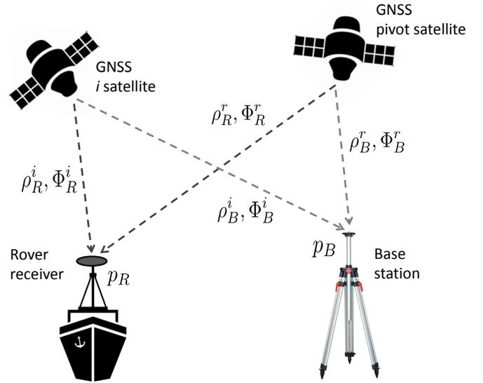
Fig. 1. RTK-principle with code and phase observations
