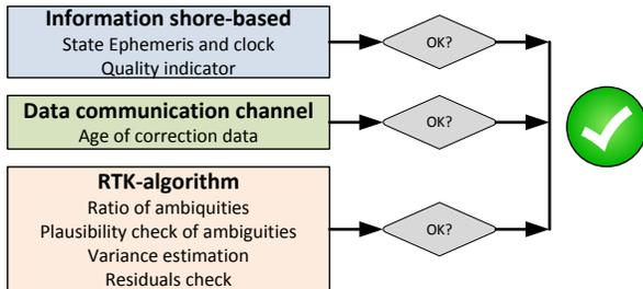
Fig. 3. Three step integrity concept
