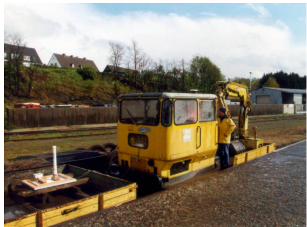
Figure 7: Train of the Schleifkottenbahn, H-field- and E-field antenna mounted on the wagon, GPS mounted on the driving cab
