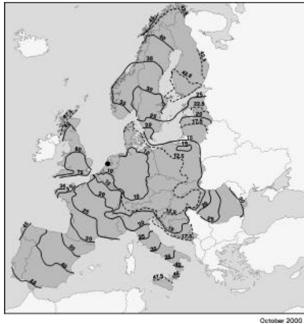
Figure 4: UELN 95)98 – Isoline of Precision [kgal . mm]
