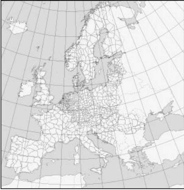
Figure 1: United European Levelling Network 1995 (UEN-95/98 – extended for Estonia, Latvia, Lithuania and Romania)
