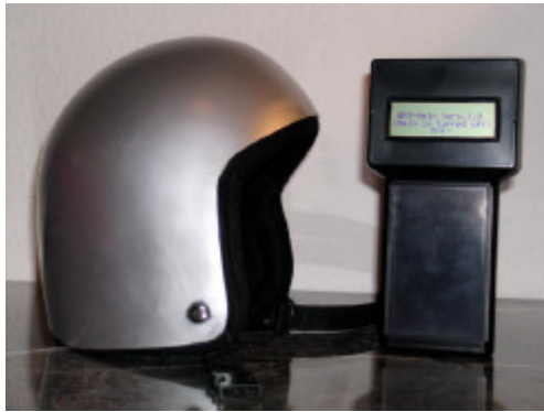
Fig 1: GPS-Helmet receiver and handheld display for receiver status information.
