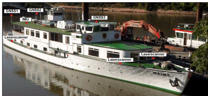
Figure 7: Vessel BS Mainz with all sensors elements
