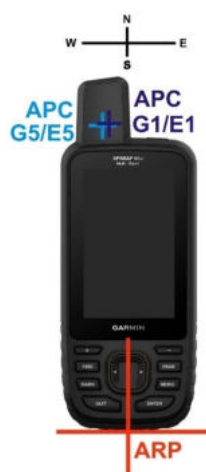
Figure 10. Depiction of the necessary specifications with regard to antenna phase center (APC) calibration: position of the antenna reference point (ARP) and azimuthal orientation of the device toward north. The mean APCs as determined by calibration are also shown.
