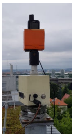
Figure 9. GPSMAP 66sr in its holder on top of the DRB2 rotational device, which enables observations in four azimuthal orientations per minute.
