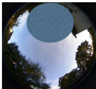
Figure 14. Limited sky visibility at the adverse observation site due to signal obstructions and the satellite visibility gap around the north celestial pole.
