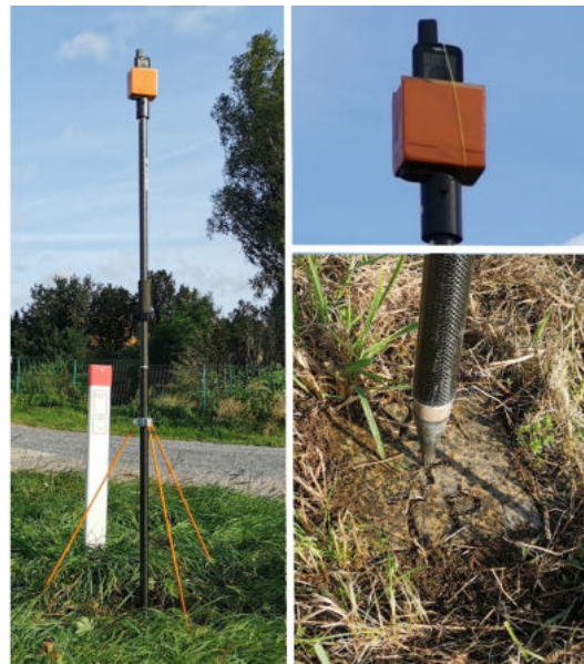
Figure 17. Receiver setup at geodetic control points on top of a 2 m pole.
