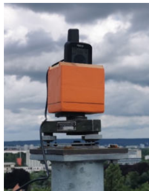
Figure 12. GPSMAP 66sr mounted on tribrach and holder for long-term observations in roof-top environment.
