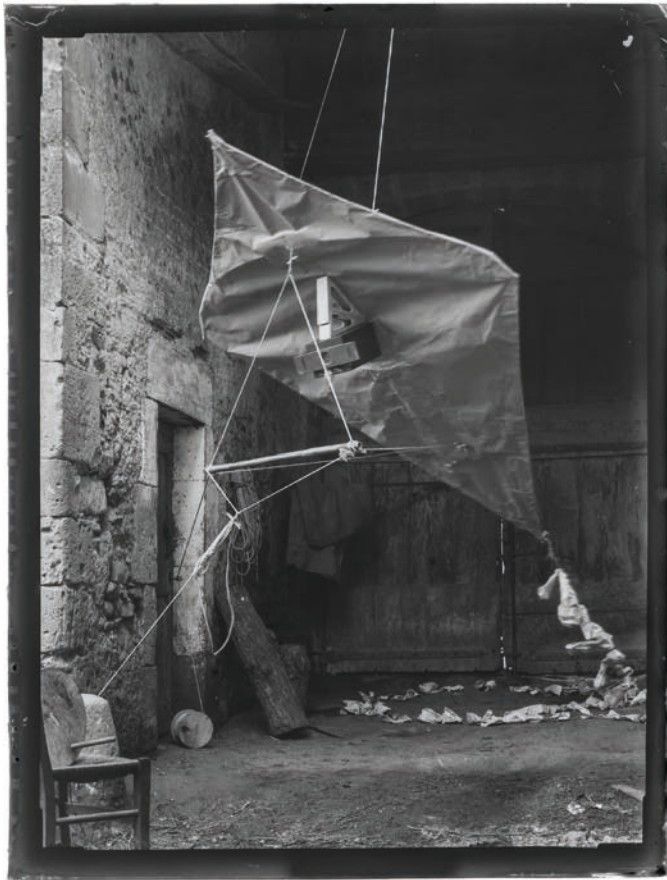
Figure 1.1-1: Wood-and-paper kite (approx. 2,5 m x 1,75 m) used by Arthur Batut for aerial photography since 1888. The wooden box camera is fitted with a simple lens and its shutter was triggered with a slow match that was lit before launching the kite. Photography by A. Batut, 1890. Image credits: Collection Espace photographique Arthur Batut/Archives départementales du Tarn.
