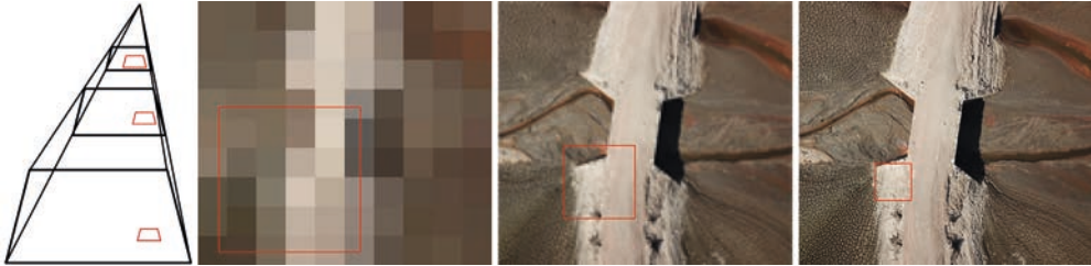
Figure 3.3-8: Applying image pyramids to improve the tracking robustness and accuracy. The highest level corresponds to the image of the lowest resolution (first image), and the base level corresponds to the image of the highest resolution (last image). The matching result at each level serves as an approximation for the next level. The kernel has the same number of pixels in each level, and therefore different areas of the scenery are covered. Note that kernel size and downsampling are not scaled accordingly in this example to enhance the visibility of changes at different levels.
