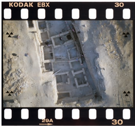
Figure 1.1-3: Scanned 35-mm slide taken with an analogue Pentax SLR camera fitted with additional fiducial marks for digital photogrammetric processing. This kite aerial photograph of archaeological excavations at Tell Chuera settlement mound, northeastern Syria, was taken by the author in 2003, the last year before digital cameras took over.
