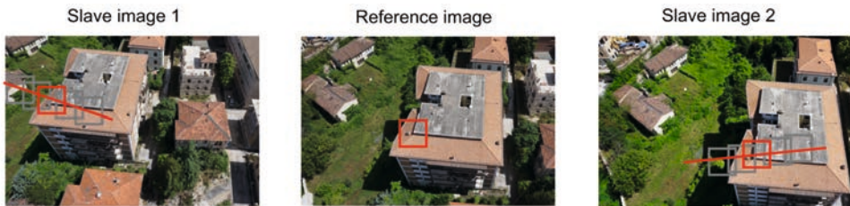
Figure 2.2-13: Epipolar geometry in a multi-image approach.
