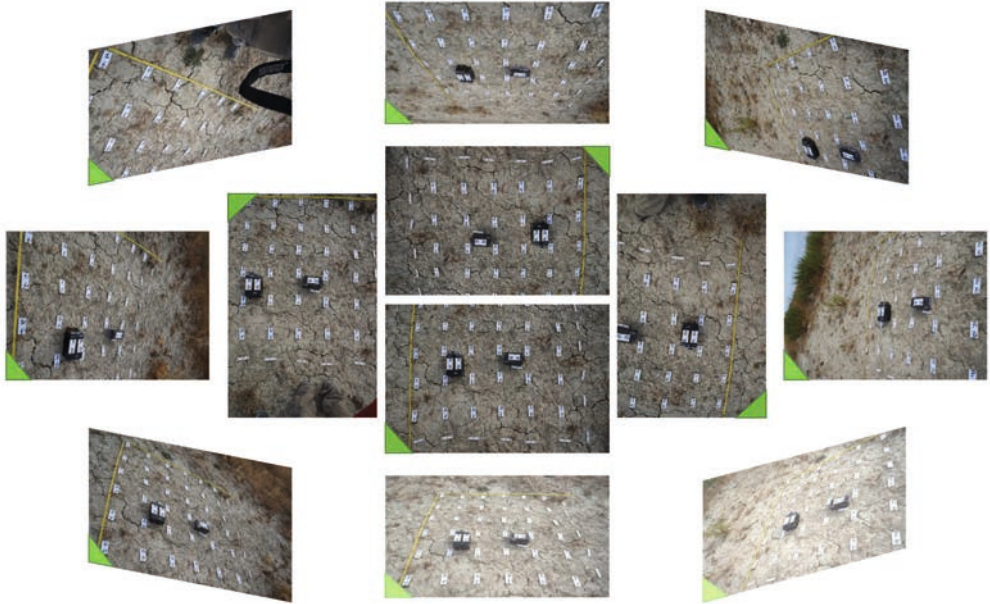
Figure 1.5-4: Example image capture arrangement for pre- or post-flight camera calibration with a temporary calibration field (for more details see Luhmann et al., 2019).
