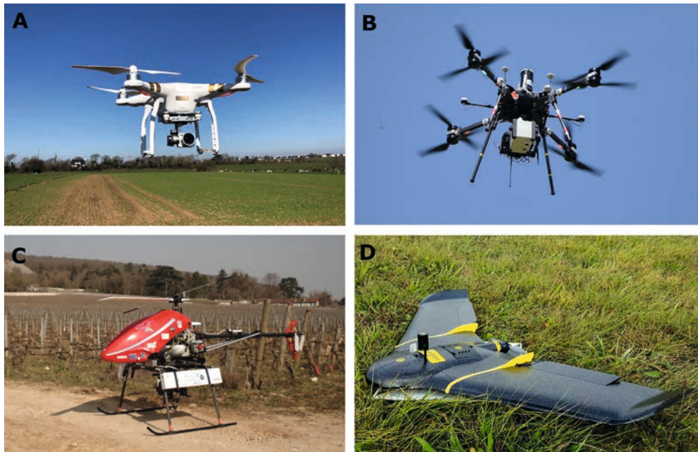
Figure 1.3-1: UAVs in use at IUEM's Ocean Geosciences Laboratory. (A) Compact RTF multirotor UAV (DJI Phantom) with an integrated image sensor. (B) Custom-built multirotor UAV in flight with its gyro-stabilized hyperspectral sensor payload in a waterproof case. (C) Custom-built helicopter UAV (190 cm rotor diameter) equipped with side instrument pods (in white), a Reflex camera, and a thermal camera synchronized with a RTK-GPS. (D) SenseFly eBee commercial RTF fixed-wing UAV with an integrated image sensor. Image credits: (A) Jérôme Ammann LGO, CNRS – UBO. (B) Christophe Prunier LGO, CNRS – UBO. (C) Philippe Grandjean Univ-Lyon1. (D) Mouncef Sedratti LGO, CNRS – UBS.
