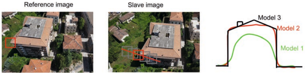
Figure 2.2-12: Multi-resolution approach in a stereo pair (please note the shorted epipolar line) and progressive reconstruction of the model from coarser (using low-resolution images) to more defined (using full-resolution images).
