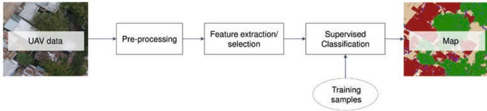
Figure 3.2-1: Diagram of the classical image classification workflow. Unless otherwise stated, all images were prepared by the authors for this chapter.
