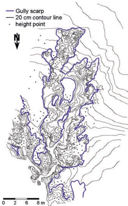
Figure 1.1-4: Left: Topographic map of Gully Oursi, Burkina Faso, created in 2002. The gully scarps, contour lines and height points were manually mapped as 3D vector data with ERDAS StereoAnalyst using a stereo-model from scanned 35-mm slides that was viewed with active shutter glasses on a stereo computer monitor. Right: TIN surface model computed from the 3D points and lines. Adapted from Marzloff et al. (2003).
