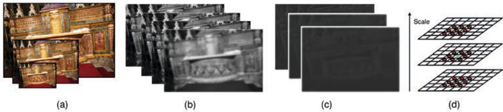
Figure 2.2-9: Example of octaves (a), image scales (b), Differences of Gaussians (c) and local extremes search across three image scales (d).
