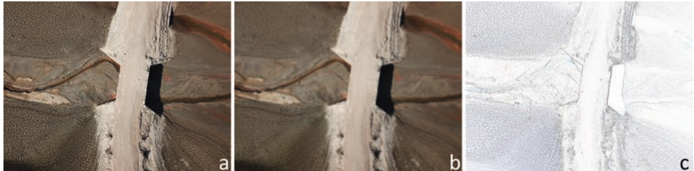
Figure 3.3-3: Different options of image filtering to reduce the impact of image noise or to increase the tracking robustness. (a) Original image. (b) Gaussian filtered image for smoothing. (c) Laplace filtered image to keep edges only for tracking.
