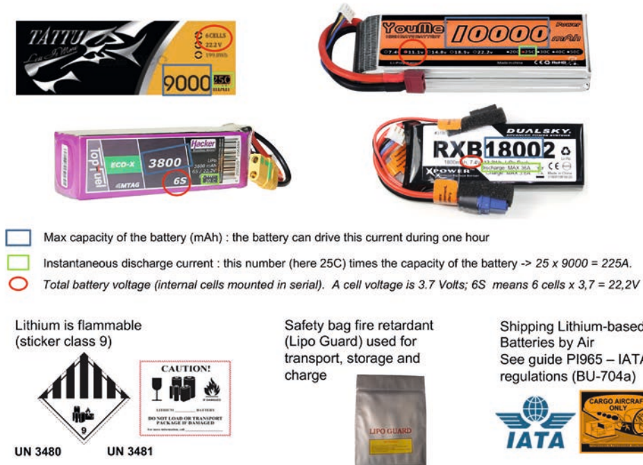
Figure 1.3-8: How to read a battery sticker.
