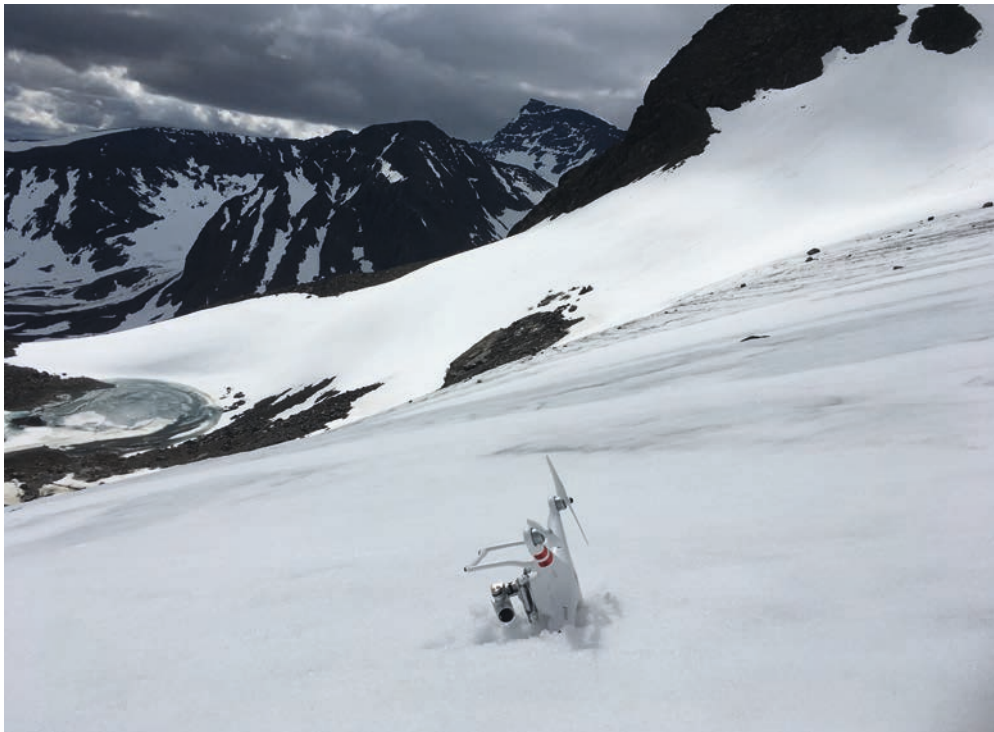
Figure 4.5.-3: Poor GNSS signals coupled with mountain winds result in more UAV take-offs than landings in cryospheric research.
