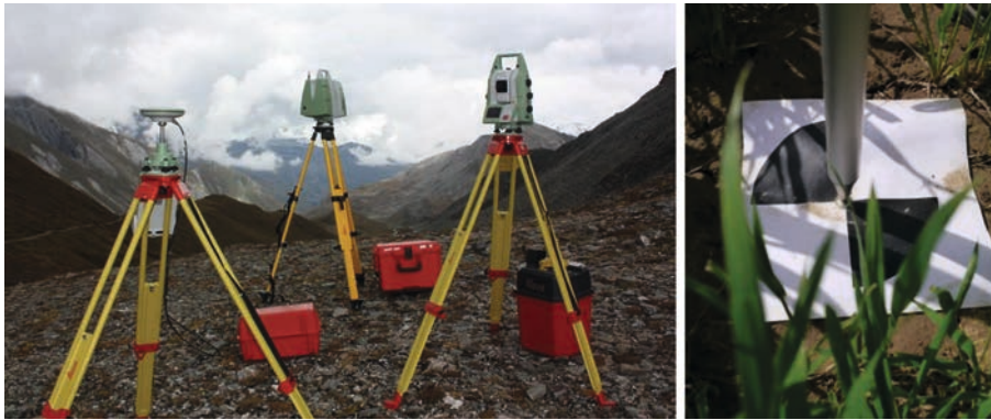
Figure 2.1-2: Left: Terrestrial Geodetic measurement equipment on tripods (from left to right: GNSS Antenna, Terrestrial Laser Scanner, Total Station). Right: Ground Control Point (GCP) for indirect georeferencing. Image credits: Christoph Holst.
