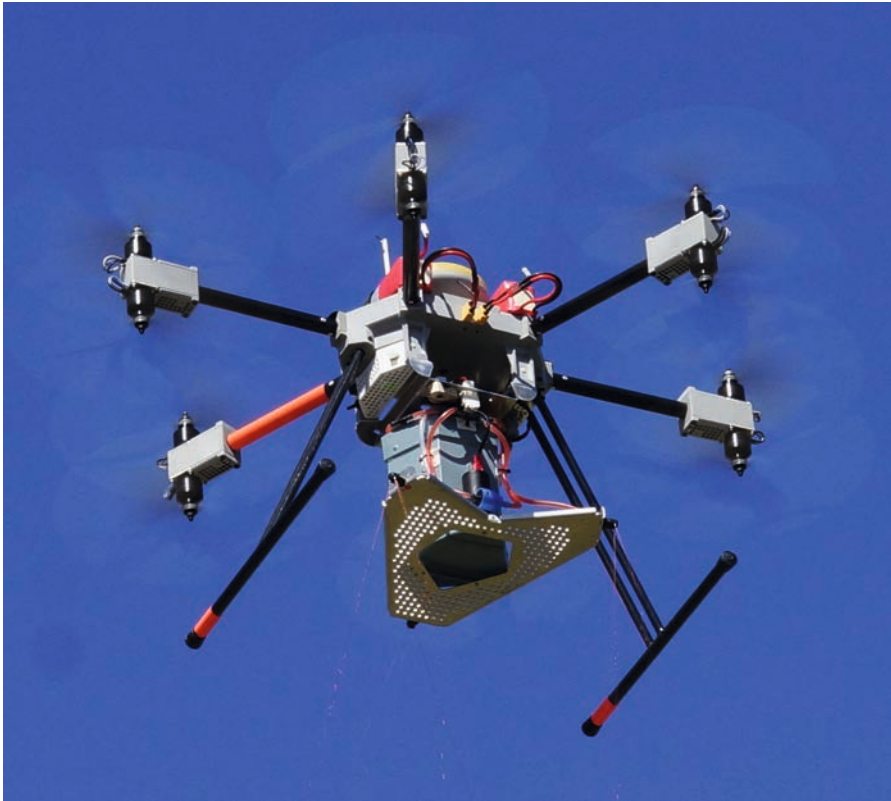
Figure 1.2-3: UAV prototype equipped with a tank for spraying application.
