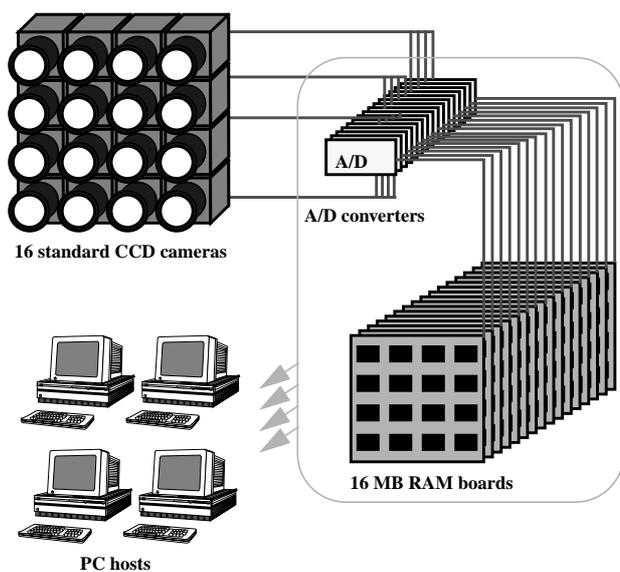
Figure 6: Cascaded 16 CCD camera system (scheme)
