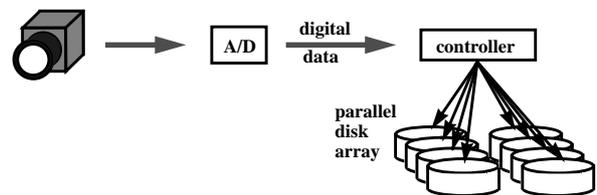
Figure 4: Parallel disk array - principle
