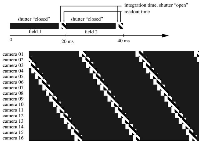
Figure 5: Phase shifted synchronization of 16 CCD cameras
