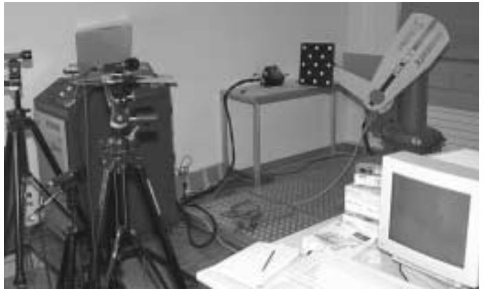
Fig. 2: Signalized robot (Stäubli Puma 500), three camera photogrammetric system
