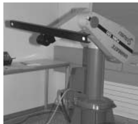
Fig. 3: Reference bar for scale definition in the automatic self calibration of the photogrammetric system
