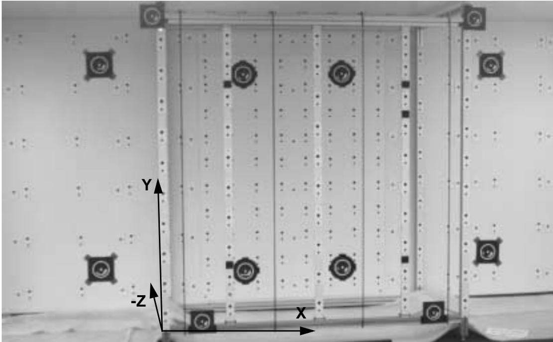
**Fig. 1: ETH camera calibration field with coded and uncoded targets**
