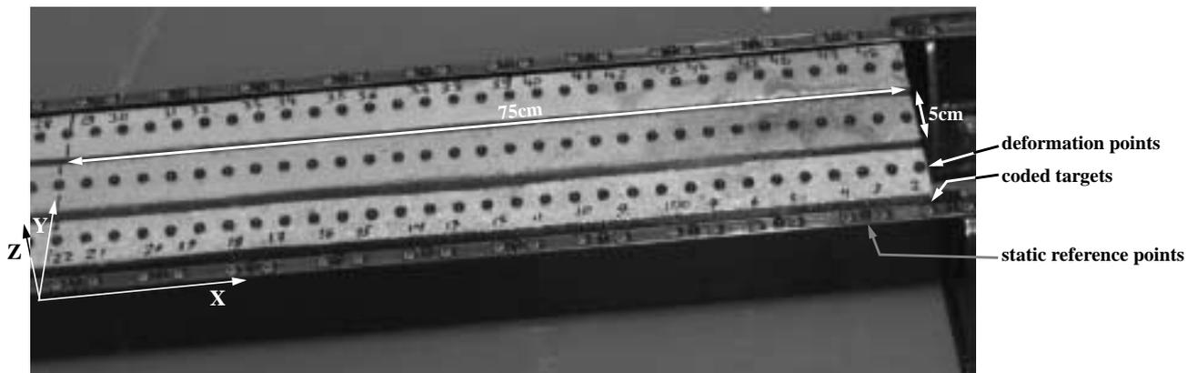
Fig. 2: Targeted concrete parts in deformation test
